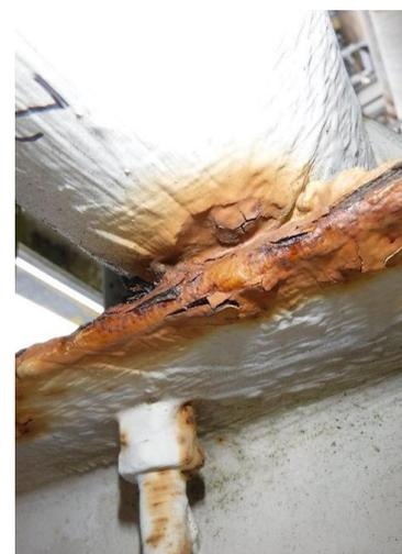
**Photograph of 2" U-bolt specimen with visible signs of corrosion at the contact point with flat beam support.**
