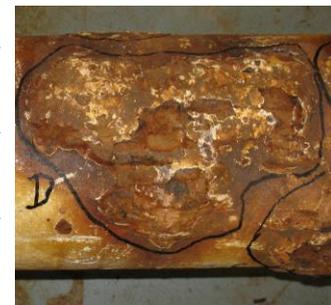
**Benchmark internal UT scan of an externally corroded area using the in-house scanner.**
