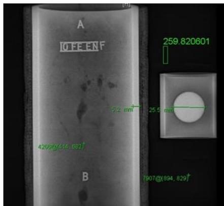
**Digital radiograph of a composite repair (courtesy CAN)**
