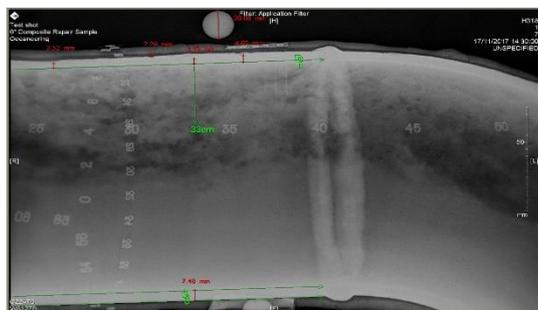
**Digital radiograph of a composite repair (courtesy Oceaneering)**
