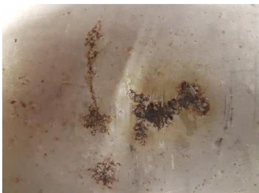
**Fine pitting and cracking on a SS component**
