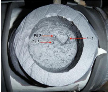
**Case study: ex-service trunnion with challenging to inspection corrosion morphology.**
