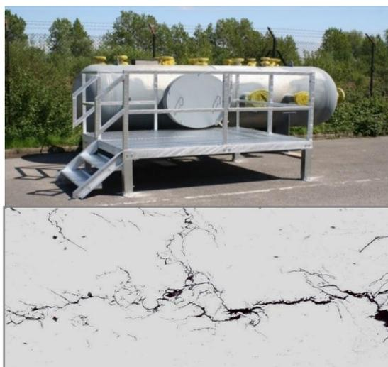
**Ex-service CRA clad vessel installed at ESR Warrington and micrograph of SCC**
