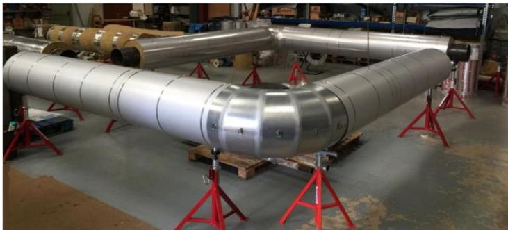
**Clad and insulated test components for trials.**
