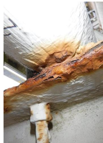
**Photograph of 2" U-bolt sample with visible signs of corrosion at the contact point with flat beam support.**
