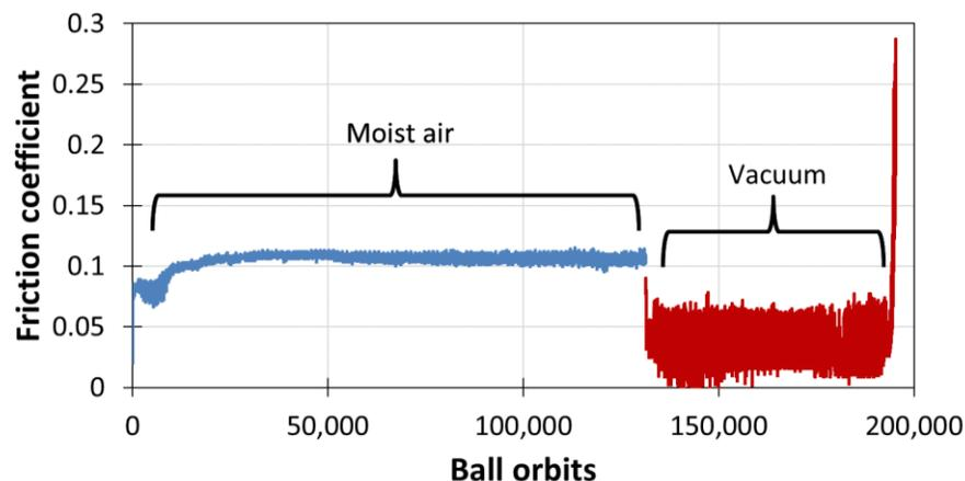
**Figure 3. Hybrid Z25/MoS<sub>2</sub> rolling in air (blue) and vacuum (red). Elevated frictional noise during vacuum running is an artefact introduced by the analysis software and is not real**
