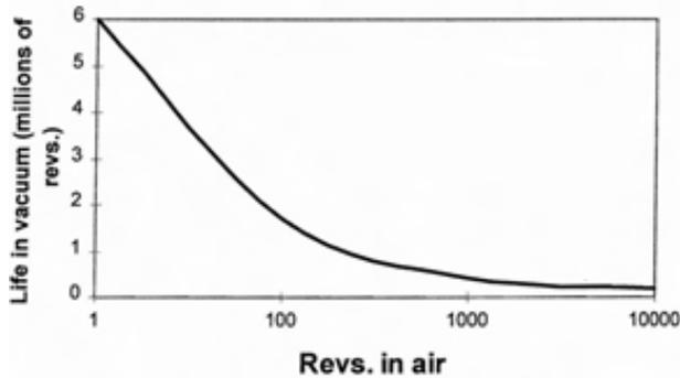
**Figure 1. Low-torque life of MoS<sub>2</sub> lubricated ED20 bearings in vacuum as a function of in-air operation prior to vacuum testing [4]**
