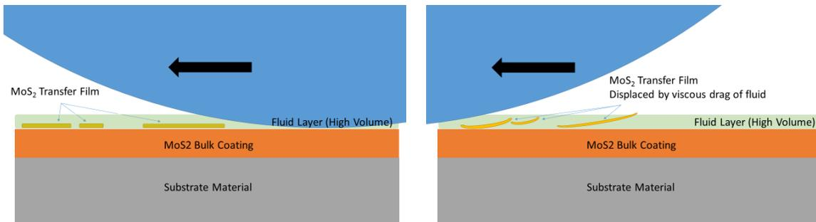
**Figure 9. MoS<sub>2</sub> transfer film formation (3<sup>rd</sup> body) of high fluid volume hybrid lubrication**
