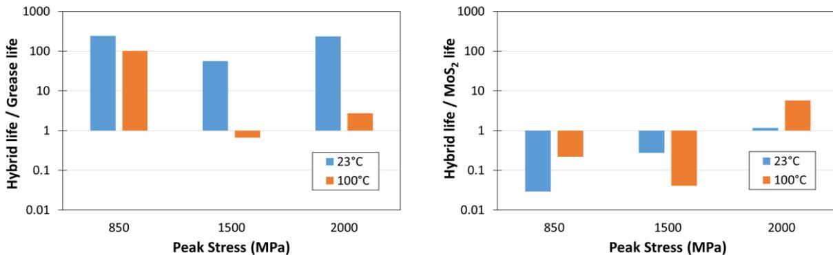
**Figure 5. Hybrid Braycote 601EF/MoS<sub>2</sub> lifetimes as a factor of Braycote 601EF-only (left) and sputtered MoS<sub>2</sub> only (right) lifetimes**
