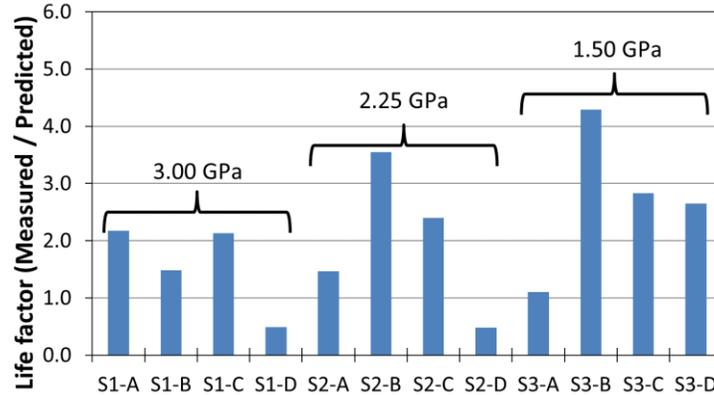
**Figure 4. Measured lifetimes of hybrid Z25/MoS<sub>2</sub> lubrication as factor of predicted life**
