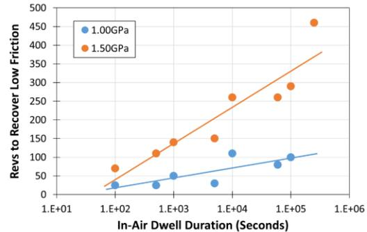
**Figure 2. PoD revs required to achieve low friction performance of sputtered MoS<sub>2</sub> under vacuum following moist air dwell period [6]**
