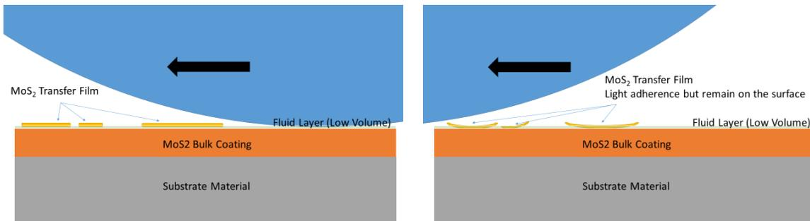
**Figure 10. MoS<sub>2</sub> transfer film formation (3<sup>rd</sup> body) of low fluid volume hybrid lubrication**
