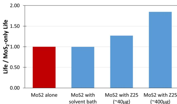
**Figure 6. Normalised performance of Z25/MoS<sub>2</sub> lubrication under vacuum**
