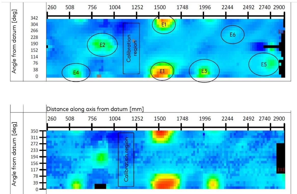
**Figure A2-34: C-scans of a 10" sch 20 stainless steel clad pipe obtained using Eddyfi Lyft with a single-element probe (lower) and the PECA™ array probe (upper) (courtesy Eddyfi).**
