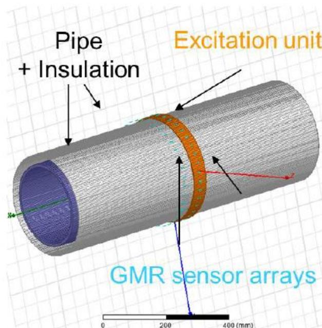
**Figure A3-21 Principle of eddy current method with GMR sensors used by Robinson Research Institute.**
