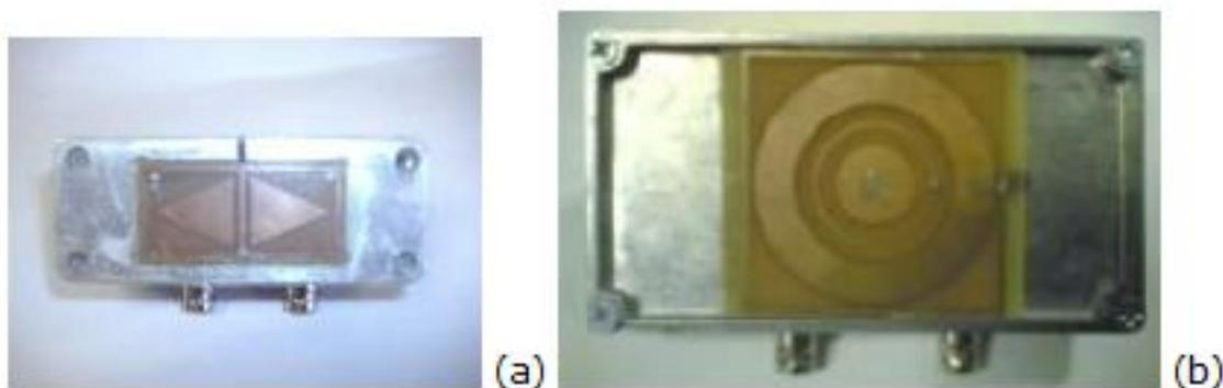
Figure A3-25 a) Photograph of a pair of triangular electrodes, mounted in a shielded metallic container. The triangular electrodes in this example were each 20 mm wide in the horizontal direction. (b) A concentric electrode design.
