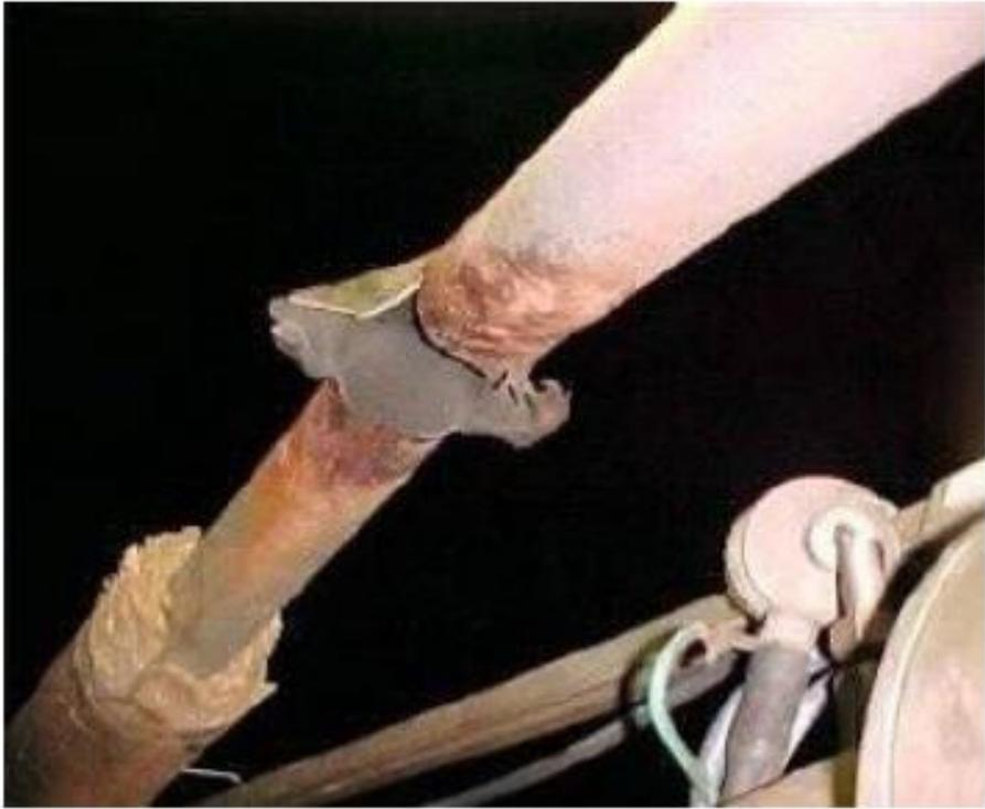
**Figure A1-3: Failure of a 4" pipe caused by CUI**
