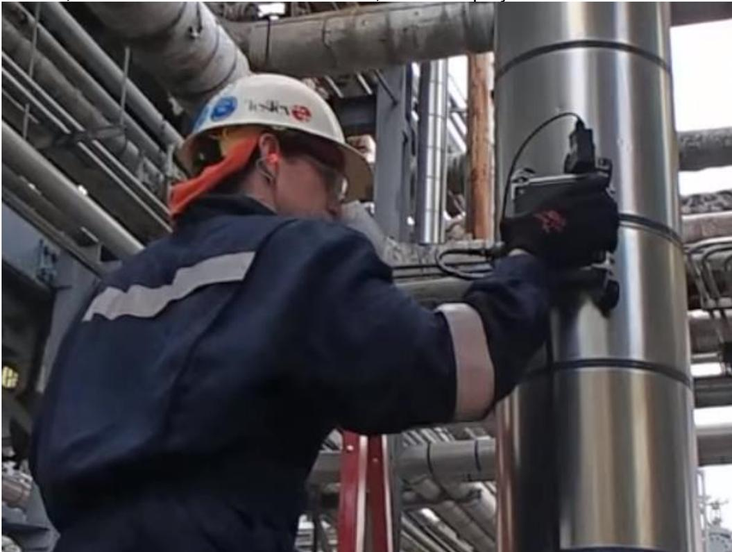
**Figure A3-20 TestEx OSET Scout scanner deployed on-site (courtesy TestEx)**
