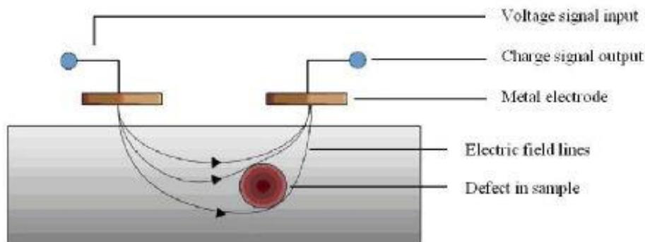
Figure A3-24 Schematic of University of Warwick capacitive imaging method for NDE.
