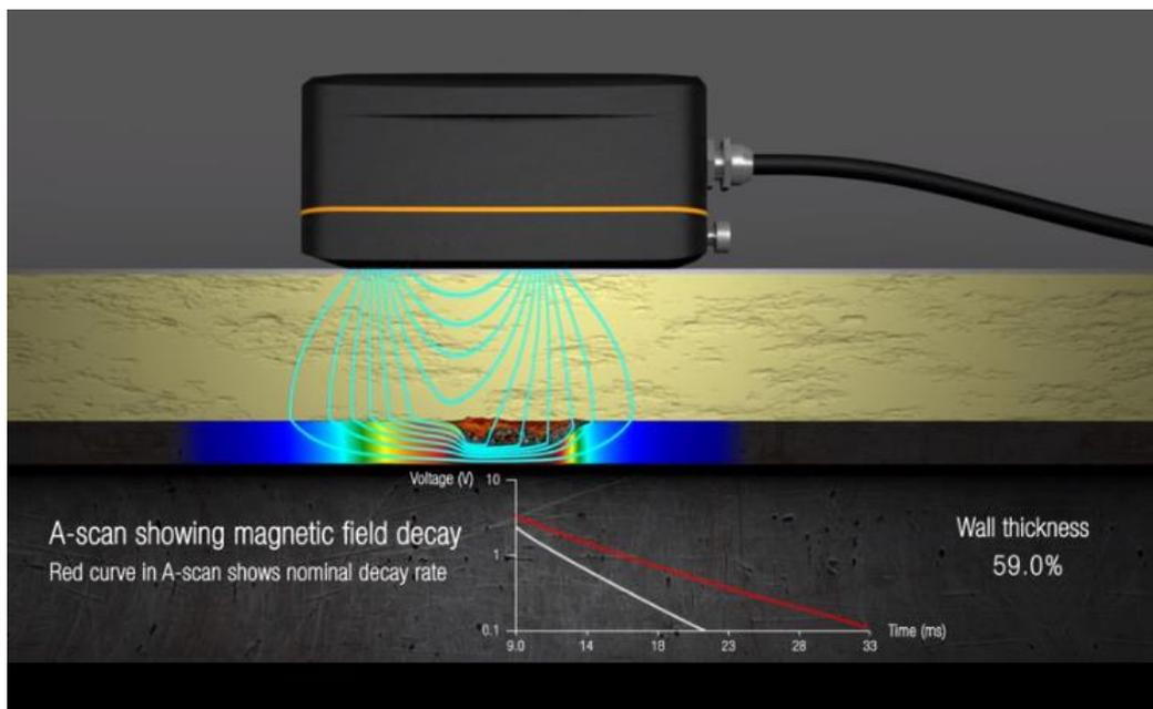
**Figure A2-31: Pulsed eddy current inspection of an area of wall loss (illustration courtesy of Eddyfi).**
