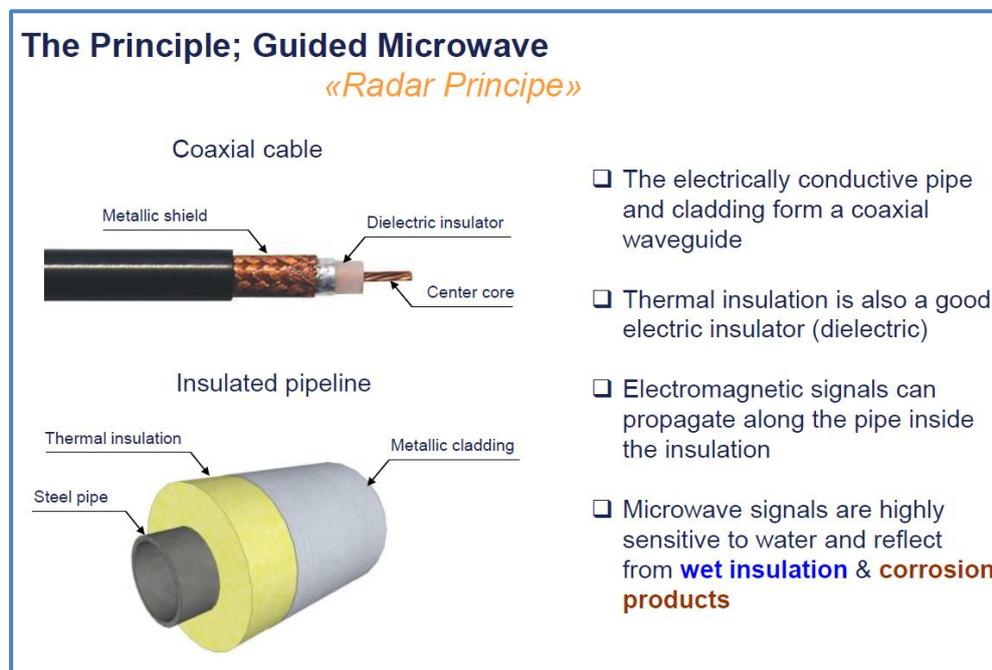
**Figure A3-6 Principle of the Guided Microwave system from ClampOn (courtesy ClampOn)**
