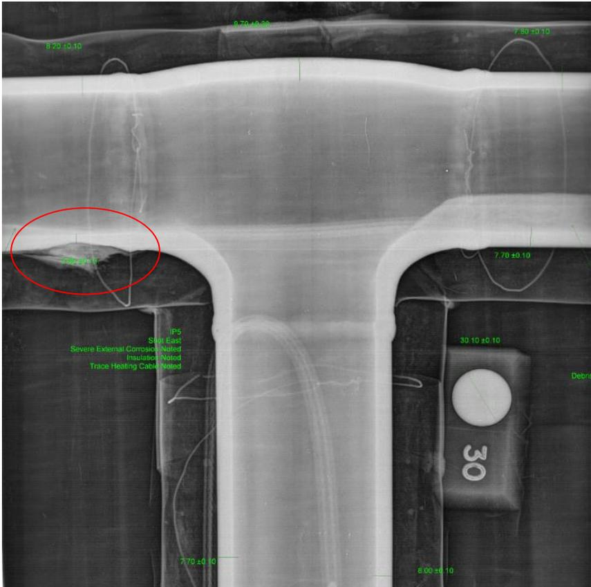
Figure A2-21: Example of combined double-wall double image and tangential radiography showing an area of CUI near a pipe tee joint (outlined in red), courtesy EM&I.
