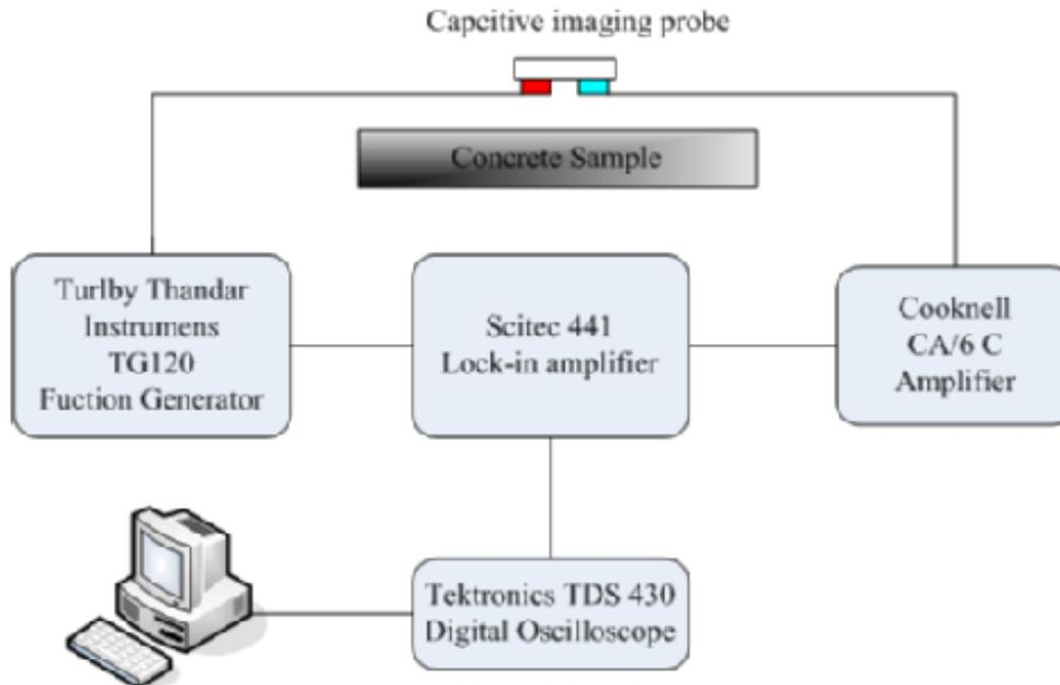
Figure A3-26 System block diagram of Capacitive imaging system.
