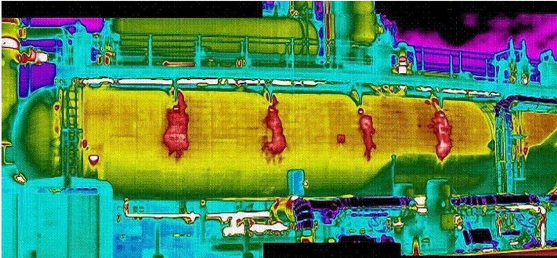
**Figure A2-5: De-Salter vessel showing water intrusion under the insulation, apparently at penetrations for the walkway along the top of the vessel (courtesy Infrared Vision).**
