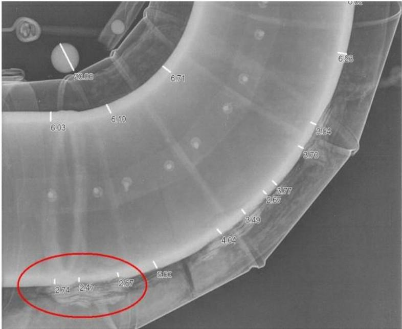
Figure A2-20: Example of combined double-wall double image and tangential radiography showing an area of CUI on a pipe bend (outlined in red), courtesy Oceaneering Ltd.
