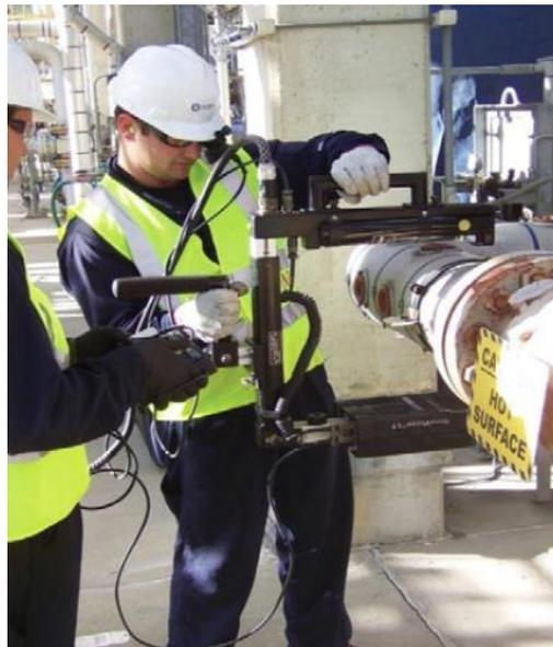
Figure A2-27: The Sentinel OpenVision real time radiography equipment being used for CUI inspection (courtesy TUV Petrochem).
