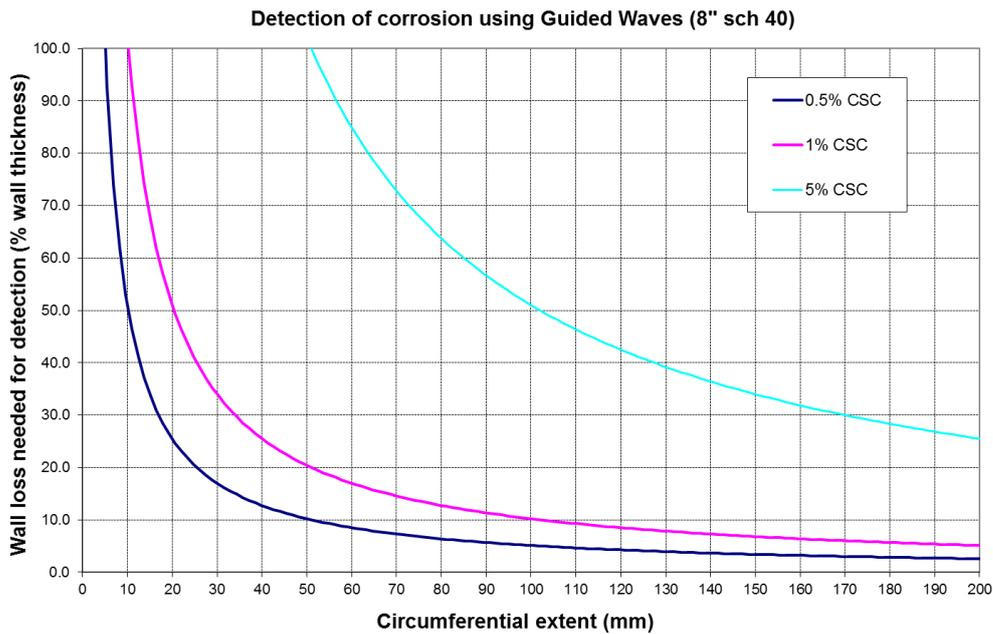
**Figure A2-14: Curves showing the wall loss (as a % of wall thickness) needed for GWT detection as a function of circumferential extent. Three different curves are shown for different detection thresholds expressed in % cross sectional change (CSC), assuming that the circumferential profile of the wall loss is elliptical (0.65 fill factor).**
