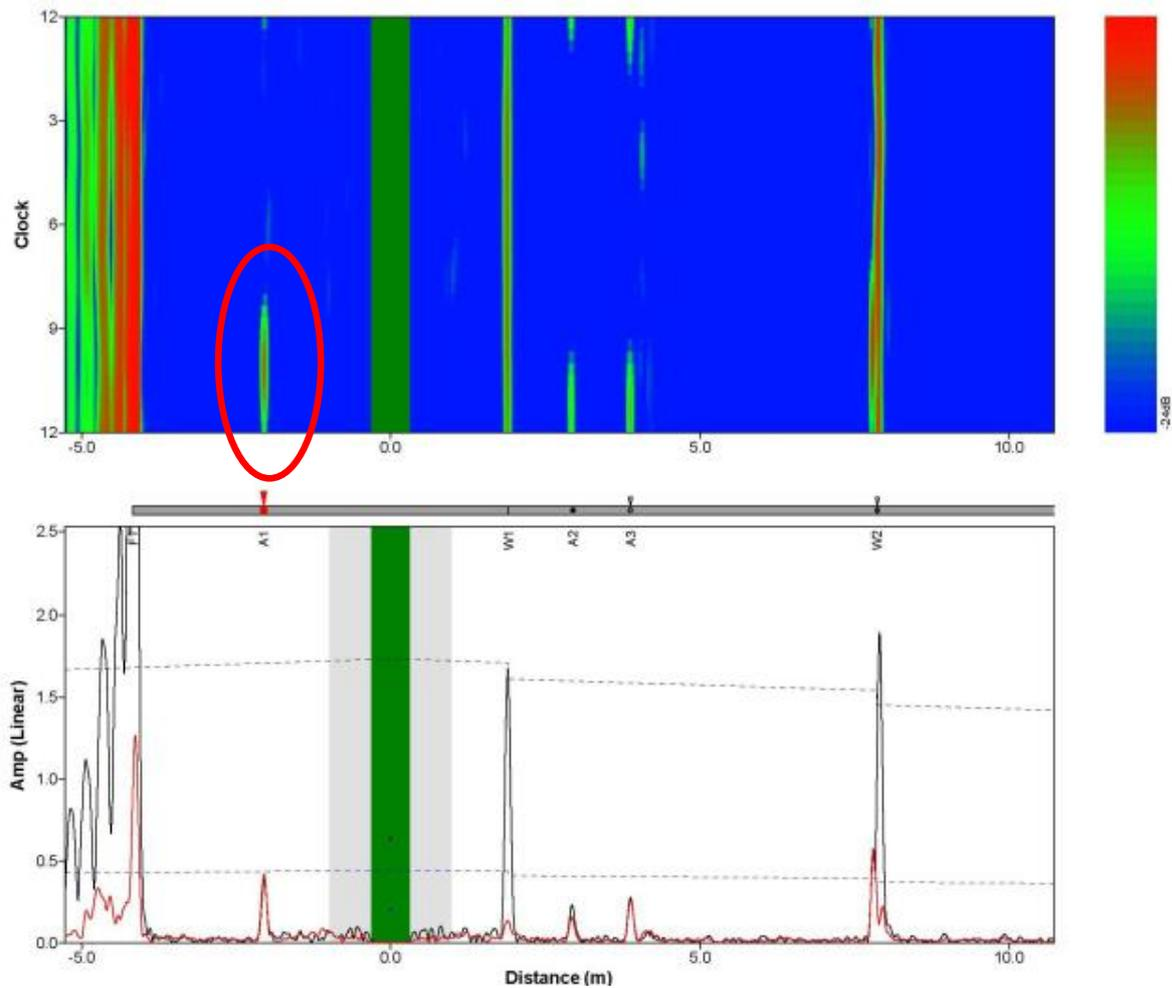
**Figure A2-13: Example of GWT results, showing both the A-Scan type trace (below), and the C-Scan type unrolled pipe display (above). The weld W1 is a symmetric feature, extending around the entire circumference, whereas the defect A1 (circled in red) is non-symmetric and localized at the 9 – 12 o'clock position. The dashed curves are DAC curves (the upper curve is the weld DAC, lower curve the call DAC) (courtesy Guided Ultrasonics Limited).**
