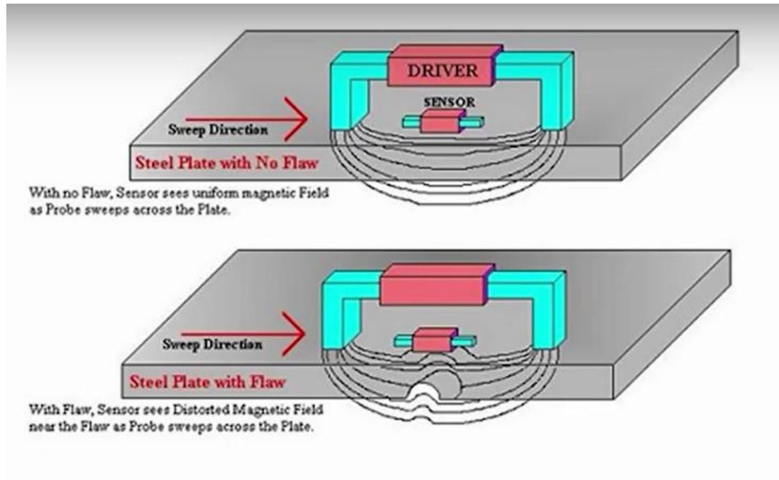
Figure A3-18 TestEx schematic of principle of LFET.
