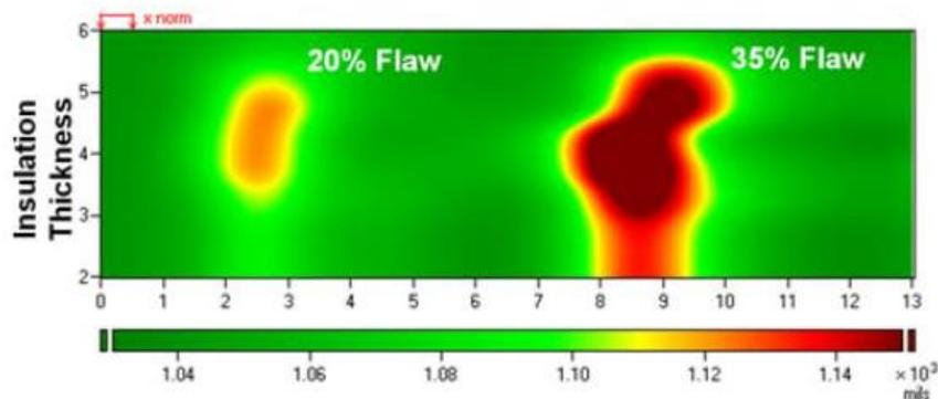
**Figure A3-17 Jentek example said to show flaws under insulation and cladding .**
