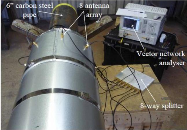
(b) Experimental setup for field test
