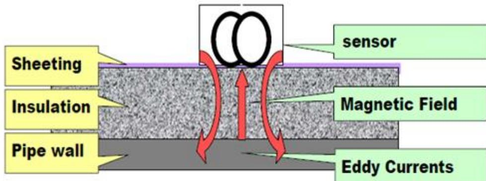
**Figure A2-30: Principle of the pulsed eddy current method for CUI inspection (illustration courtesy of ApplusRTD).**
