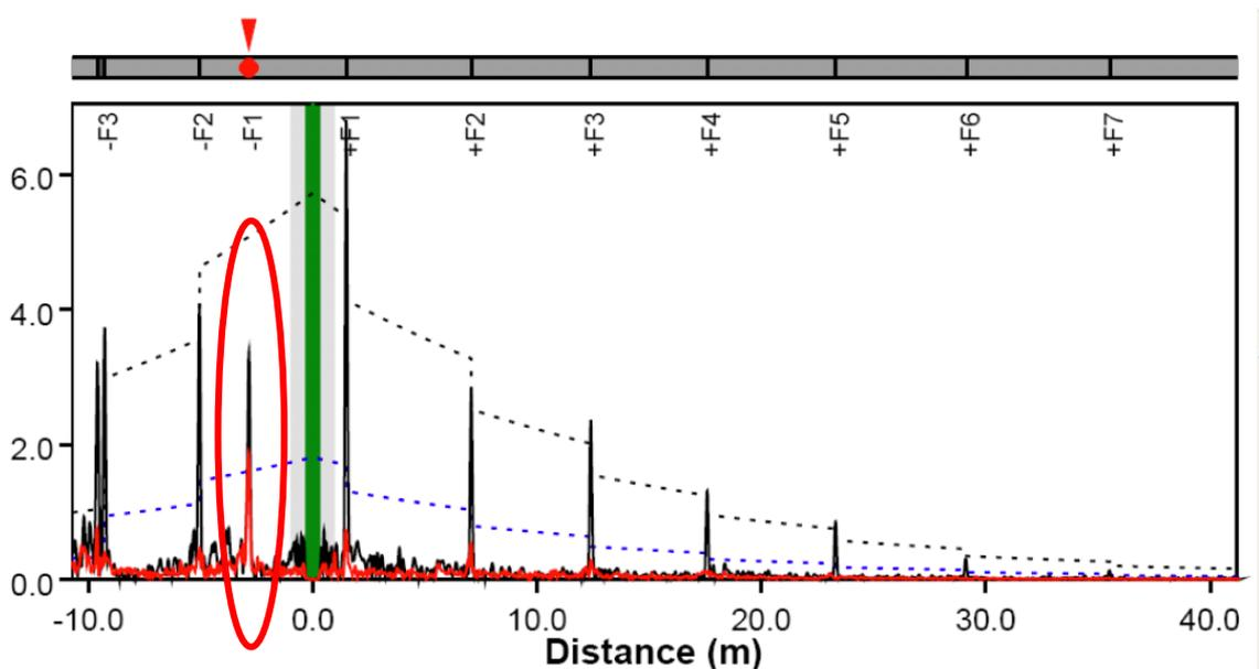
**Figure A2-16: Example of GWT data showing (in red) CUI detected and verified in a 4" pipe (courtesy Guided Ultrasonics Limited).**
