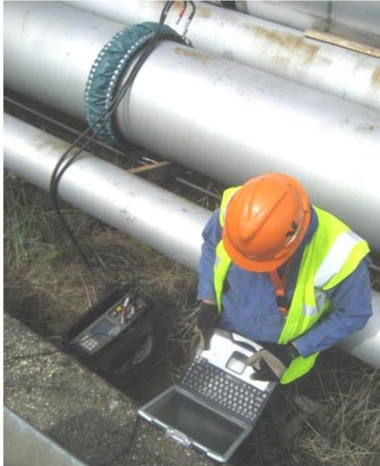
**Figure A2-12: Equipment for GWT with inflatable sensor ring attached to an un-insulated section of pipe (courtesy Guided Ultrasonics Limited).**
