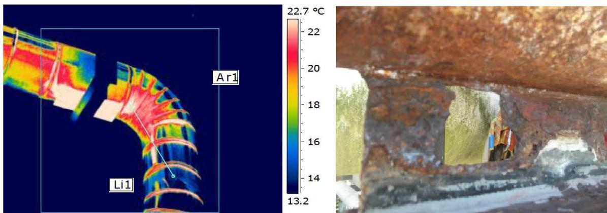
**Figure A2-7: An example of an area of corrosion found during the thermography site trial. The infrared image is shown on the left, and photographs of the corresponding insulation-stripped area is on the right. The 8" pipe was found to have a remaining WT of < 4mm.**
