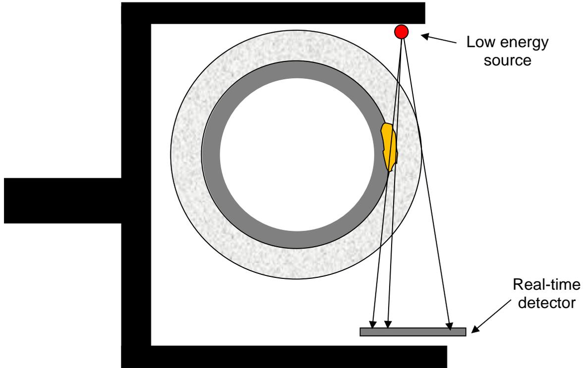
Figure A2-26: Schematic of real time radiography for CUI inspection.
