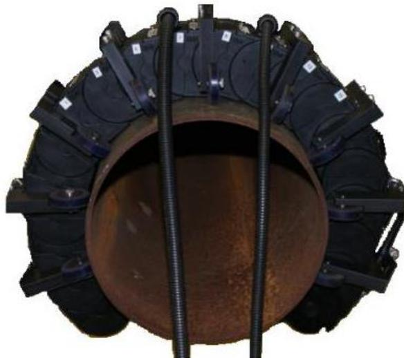
Figure A2-35: The Russell NDE bracelet probe, as applied to a pipe.
