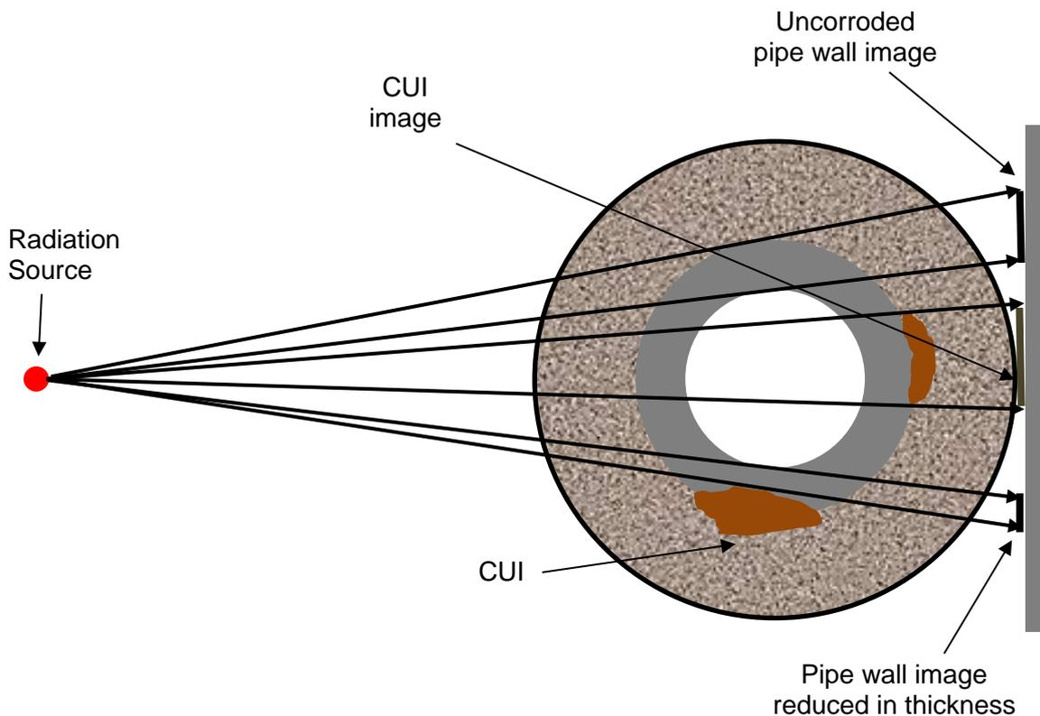
**Figure A2-18: Schematic of combined double-wall double image (DWDI) and tangential radiography for CUI inspection.**
