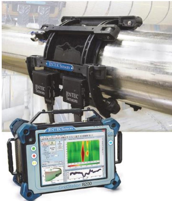
Figure A3-16 Jentek MWM technology for CUI scanning from their website (<http://www.jenteksensors.com/>).
