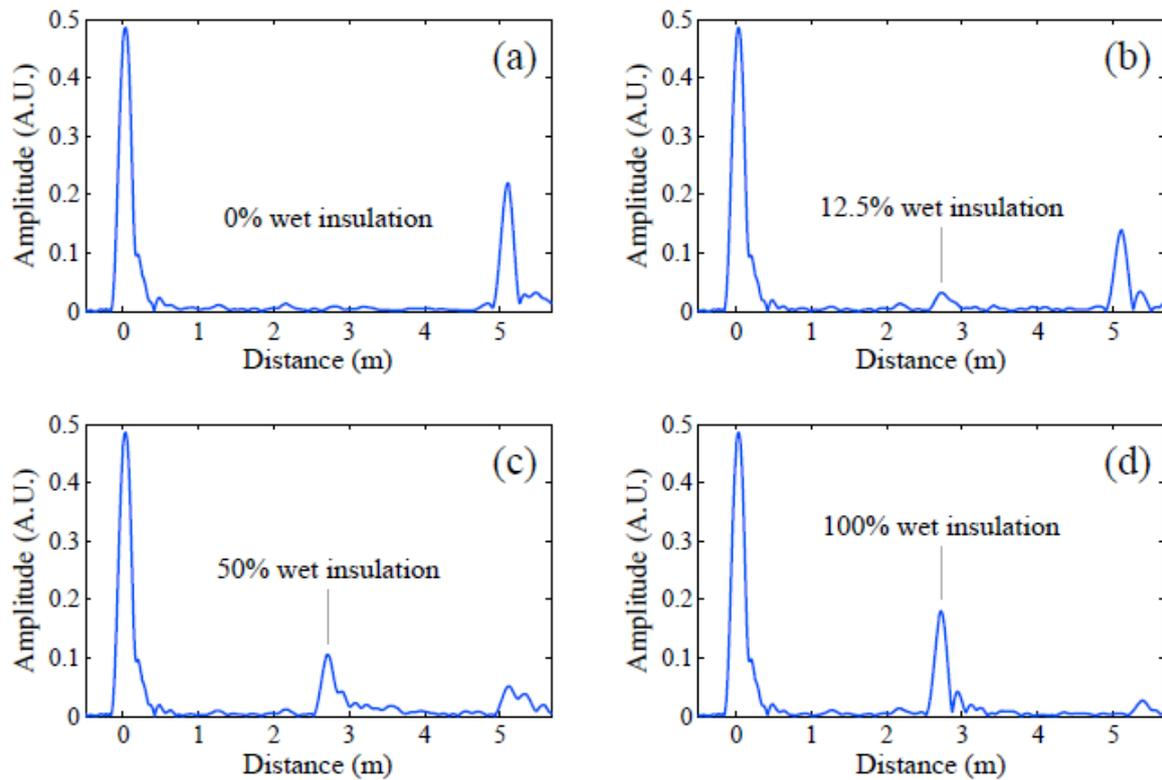
**Figure A3-5** Four examples of signals from the field tests: (a) no wet insulation; (b) one section of wet insulation, equivalent to 12.5% cross-sectional extent; (c) four wet insulation sections, equivalent to 50% cross-sectional extent; and (d) all eight wet insulation sections, equivalent to 100% of the cross-section of the waveguide annulus occupied by wet insulation
