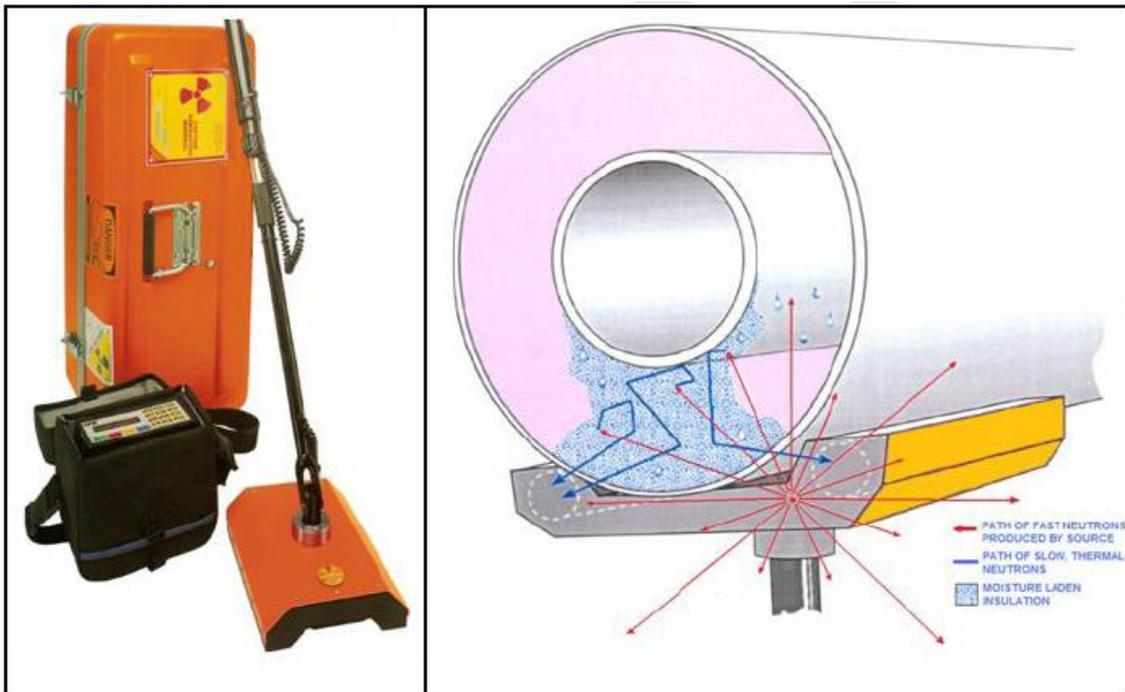
**Figure A2-9: Photo of the Hydrotector system (left) and principle of operation (right).**
