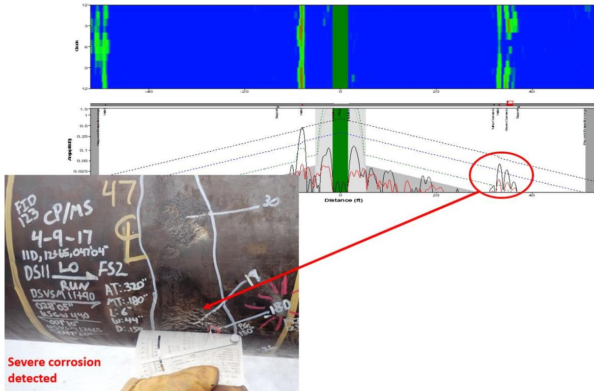
**Figure 8-5: GWT data (top) and corresponding area of CUI (bottom), confirmed after removal of the insulation.**
