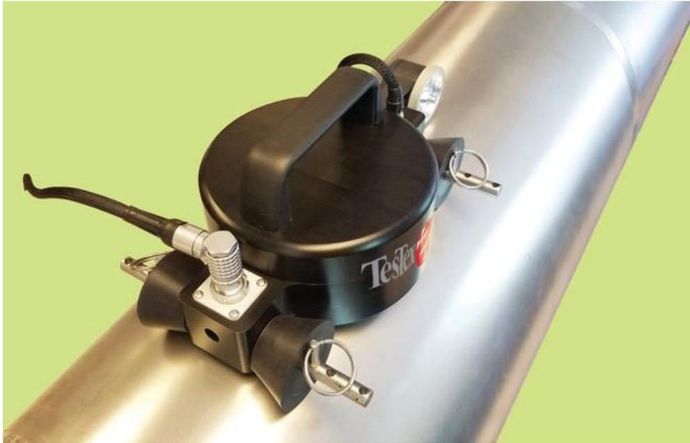
**Figure A3-19 TestEx OSET Scout scanner for CUI inspection (courtesy TestEx)**
