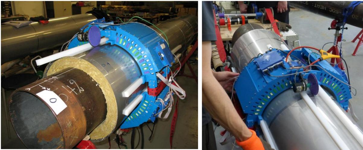
**Figure A3-22 Robinson Research Institute GMR scanner on a 10" pipe with 50mm insulation.**
