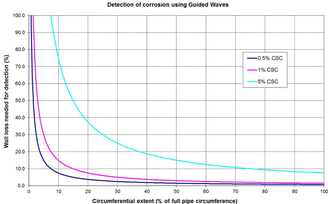
**Figure A2-15: Curves showing the wall loss (as a % of wall thickness) needed for GWT detection as a function of circumferential extent as a % of the pipe circumference. Three different curves are shown for different detection thresholds expressed in % cross sectional change (CSC).**
