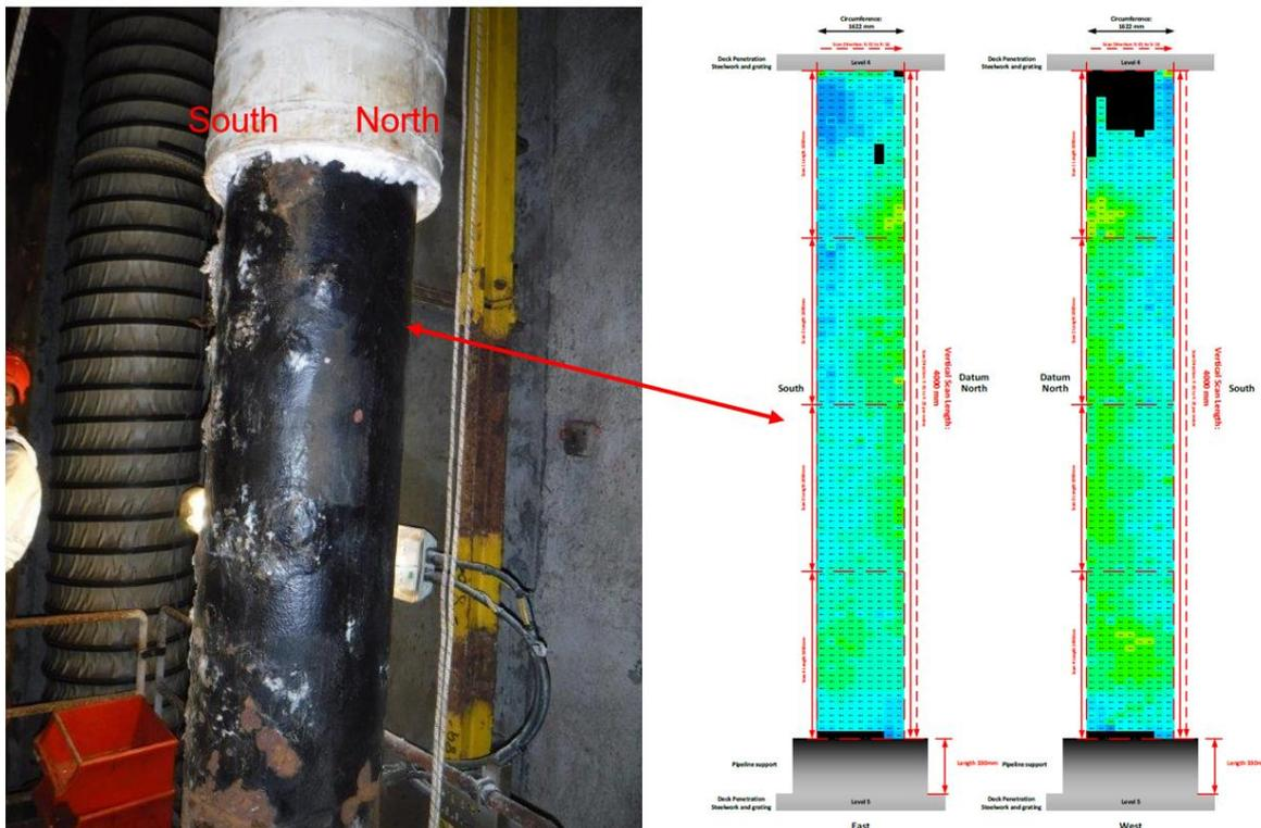
**Figure 8-12: Riser with some insulation removed (left) and corresponding PEC scan data (right).**
