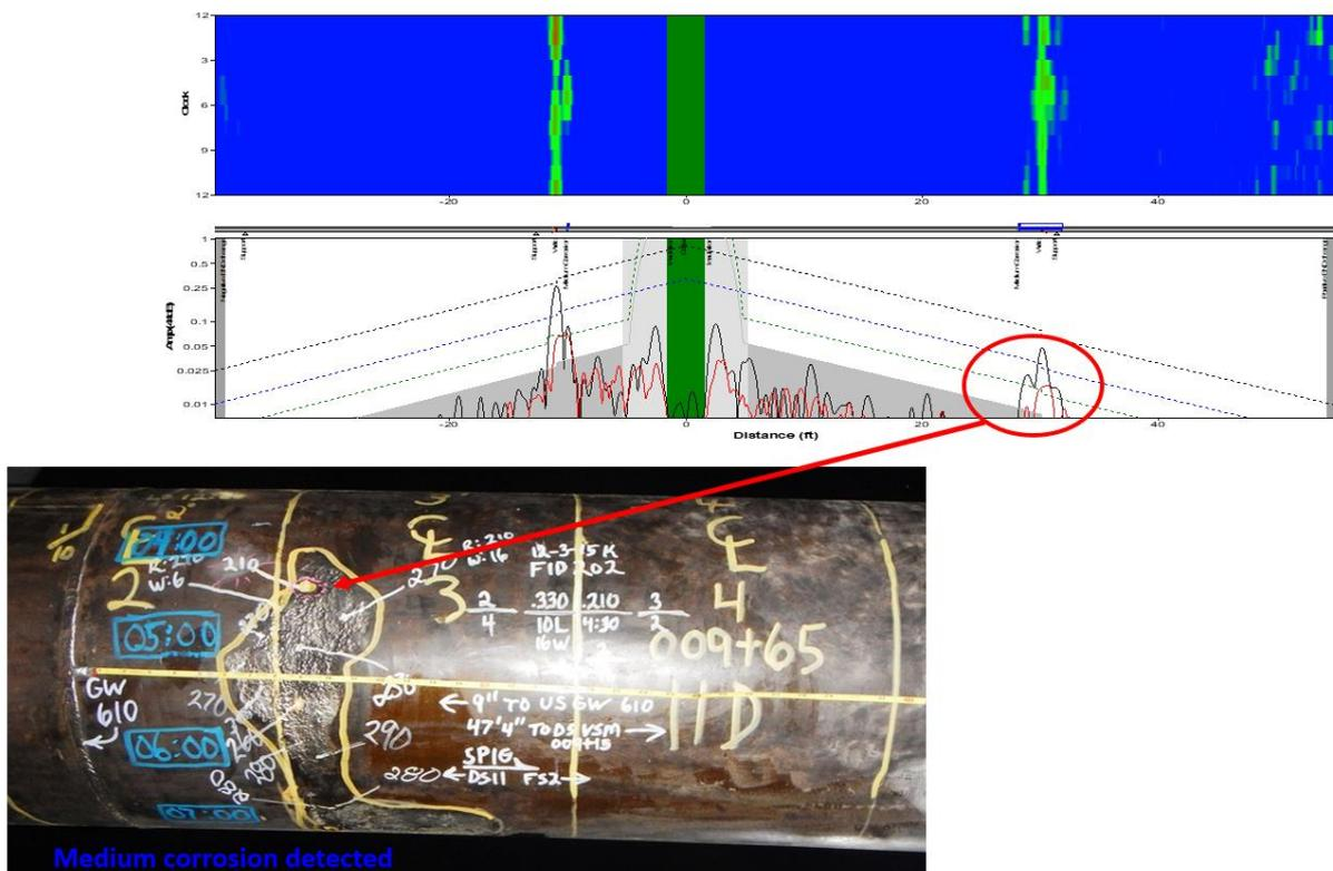
Figure 8-3: GWT data (top) and corresponding area of CUI (bottom), confirmed after removal of the insulation.
