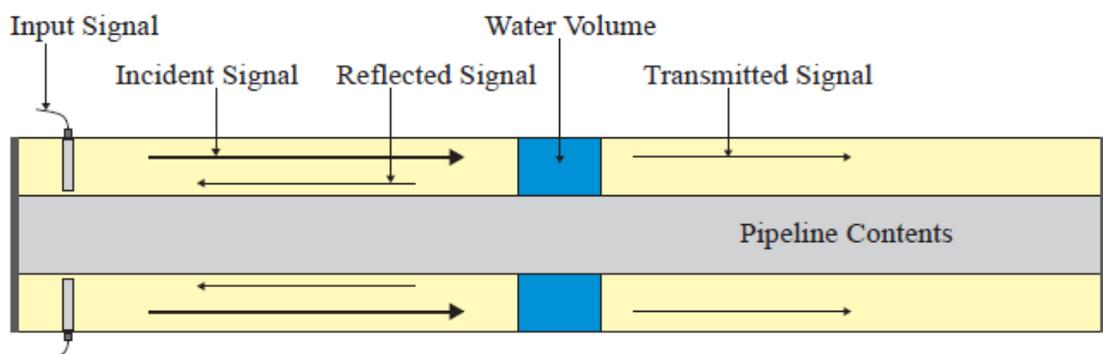
**Figure A3-3 Principle of guided microwave method**
