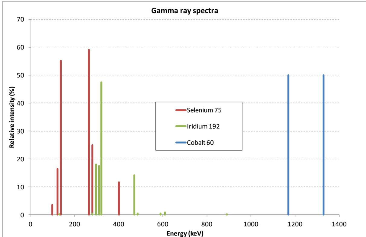
**Figure A2-17: Energy spectra of the different isotope sources used for industrial radiography.**
