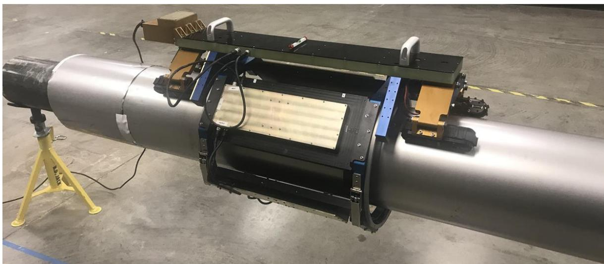
**Figure A3-15 Updated (2020) Exxam Systems automated scanner (courtesy Exxam Systems).**
