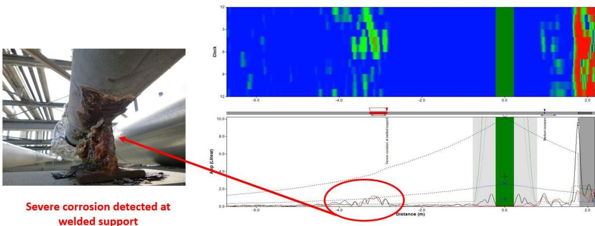
**Figure 8-2: GWT data (right) and corresponding corrosion found at the support (left), after removal of the insulation.**
