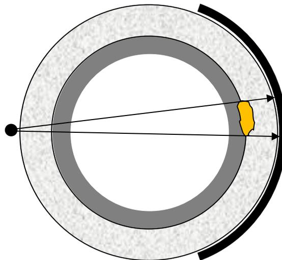
**Figure A2-25: Schematic of double-wall single image radiography for CUI inspection.**
