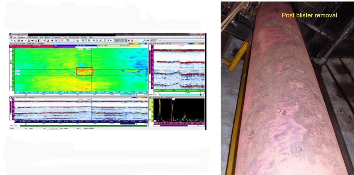
**Figure 8-14: Riser after removal of the corrosion product (right) and (left) the 0° PA scan corresponding to the minimum remaining wall thickness position.**
