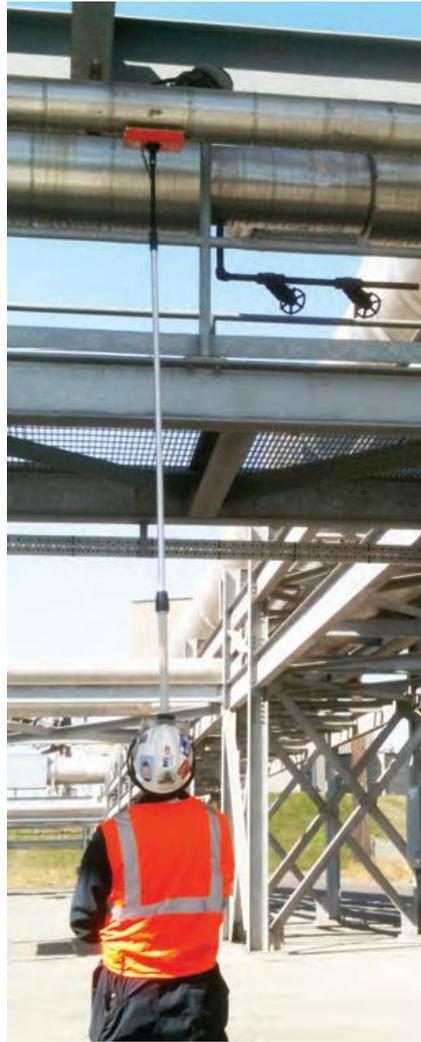
**Figure A2-10: Hydrotector system being used for CUI inspection.**
