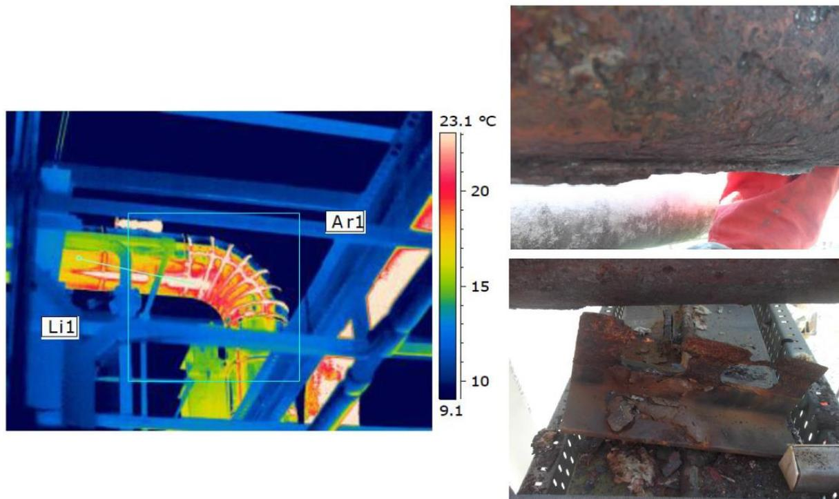
**Figure A2-8: An example of an area of corrosion found during the site thermography trial. The infrared image is shown on the left, and photographs of the corresponding insulation-stripped area is on the right. The 8" pipe was found to have a remaining WT of < 3.7mm.**
