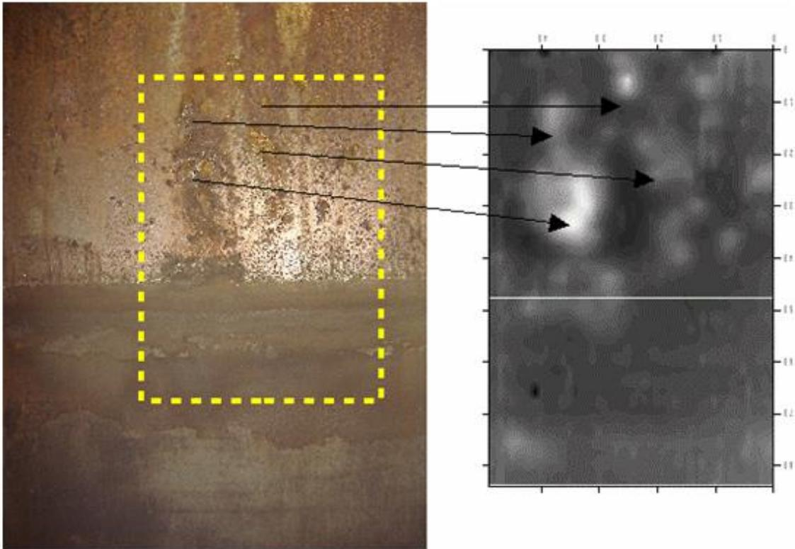
**Figure A3-27 (a) Photograph of slightly corroded steel sample. (b) Capacitive image of the same sample, with corroded areas indicated.**
