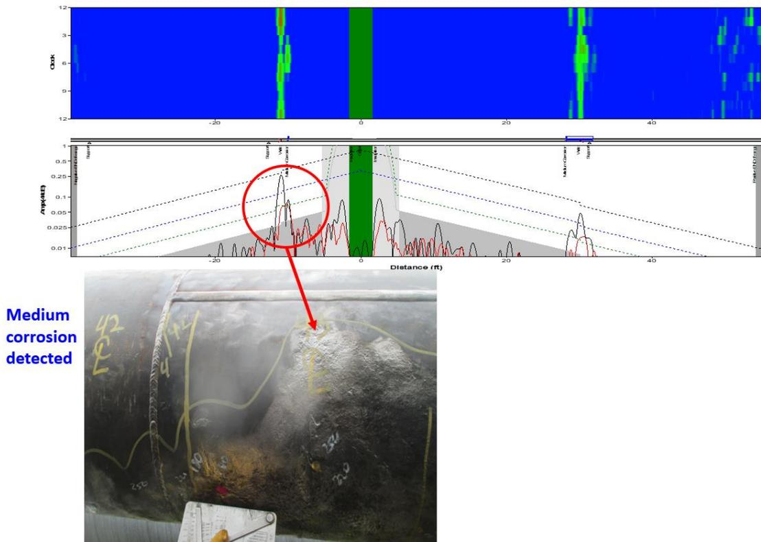
**Figure 8-4: GWT data (top) and corresponding area of CUI (bottom), confirmed after removal of the insulation.**
