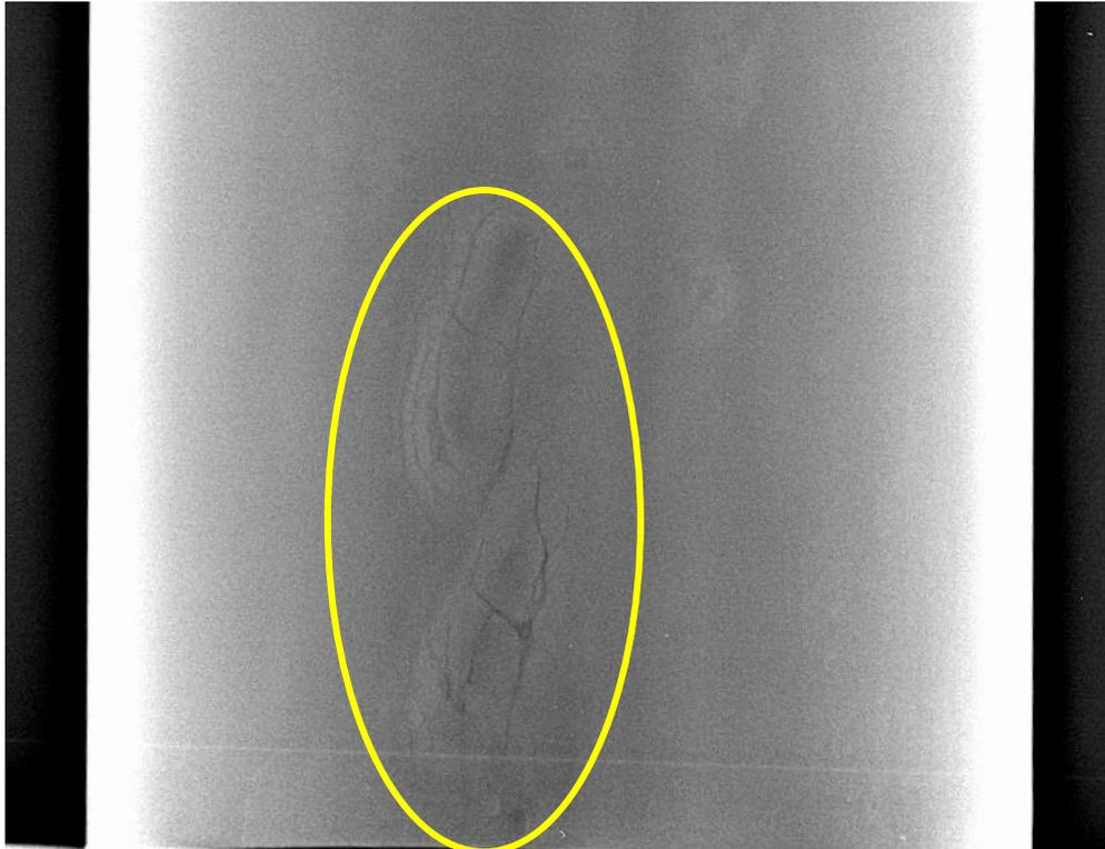
**Figure A2-22: DWDI image showing presence of external corrosion and associated corrosion product – note the overall low contrast despite the wall loss due to the corrosion being about 75% of the wall thickness, caused by the “infilling” effect of the corrosion product.**
