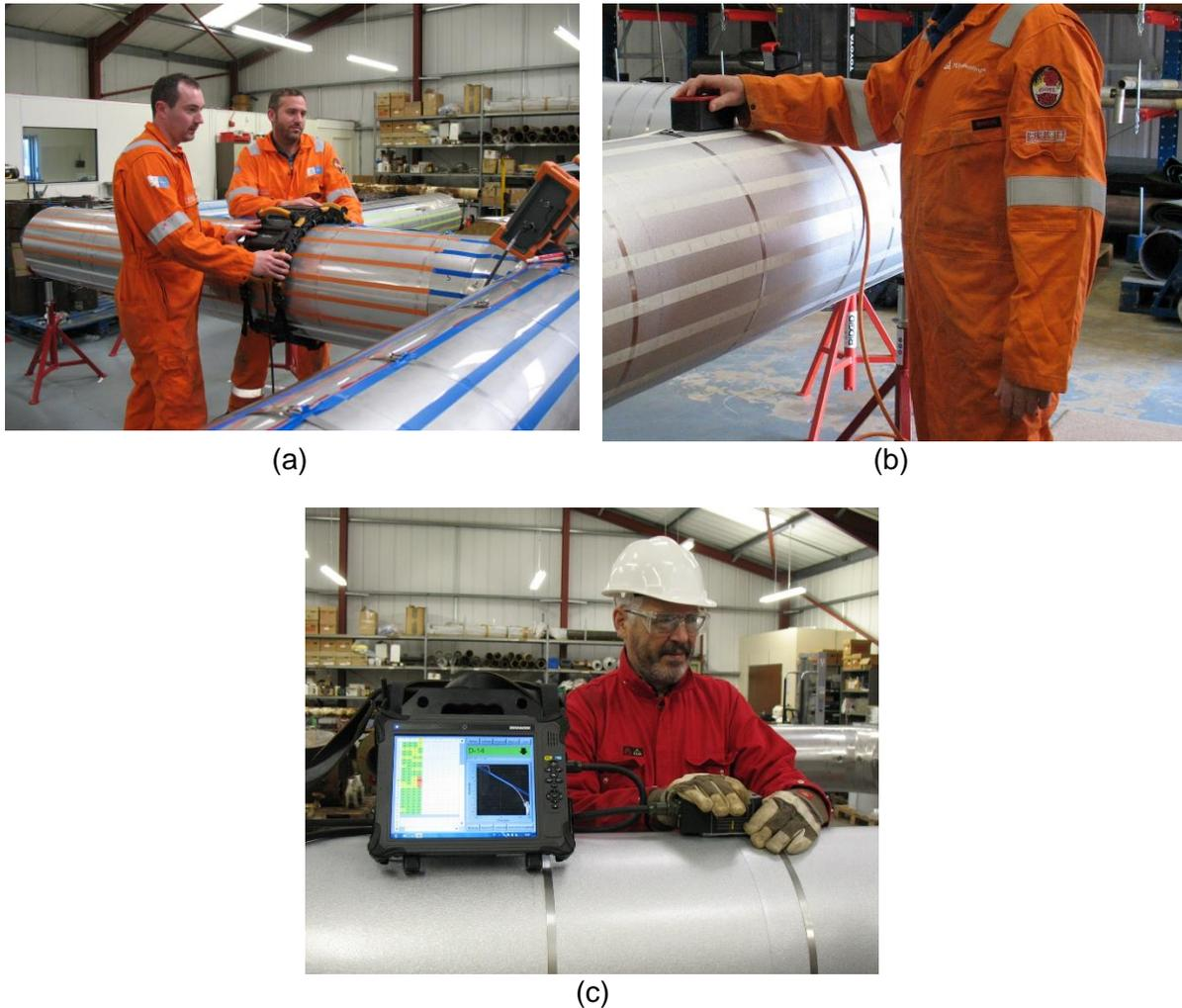
**Figure A2-33: Examples of PEC equipment being operated in the 2018/19 HOIS/OGTC CUI trials: (a) Eddyfi Lyft PECA™ array, (b) TUV Rheinland Sonovation Sonopec and (c) Maxwell NDT PECT.**
