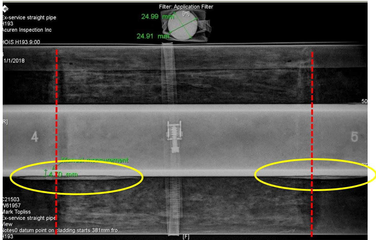
Figure A2-24: Digital radiograph obtained with an Ir 192 source and DDA. Two areas of CUI are highlighted and the extent of a wet section of insulation is indicated by the red vertical lines.
