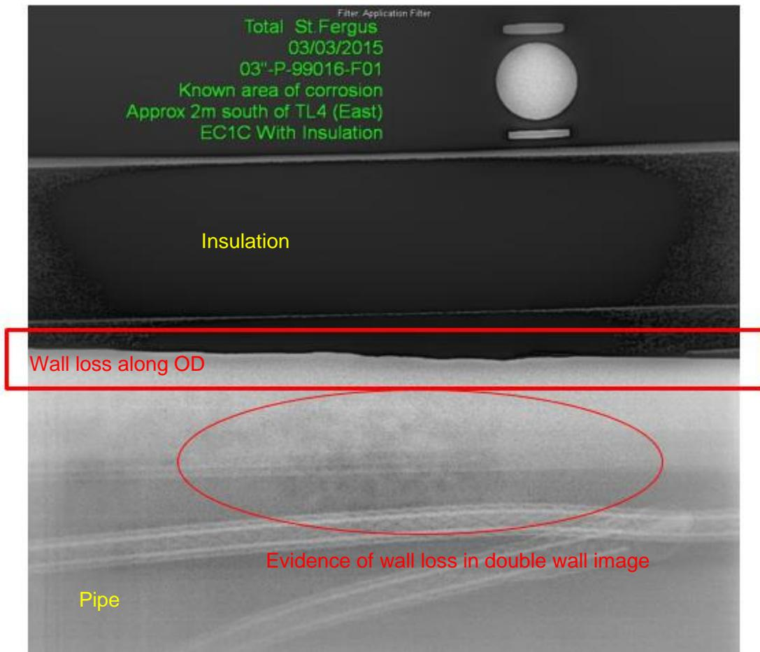
**Figure A2-23: An image of CUI taken with the flash radiography method. The corrosion can be seen within the red areas. The rectangular area shows clear corrosion on the edge of the pipe; the ellipse surrounds a darker, speckled area indicative of corrosion.**
