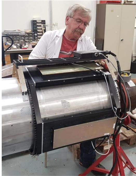
**Figure A3-14 Exxam systems scanner on a 10” pipe with 100mm insulation, as part of the HOIS/OGTC CUI trials.**
