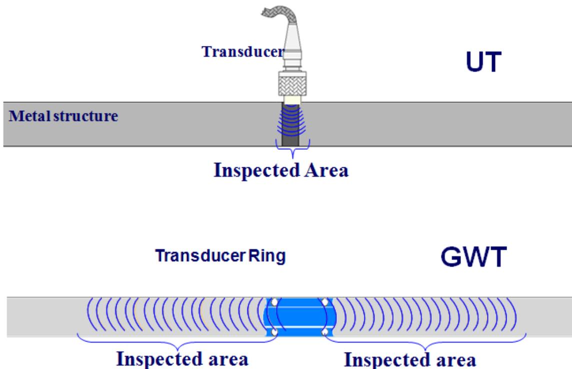
Figure A2-11: Operation of guided wave testing (GWT) compared with 0° pulse-echo UT (courtesy Guided Ultrasonics Limited).
