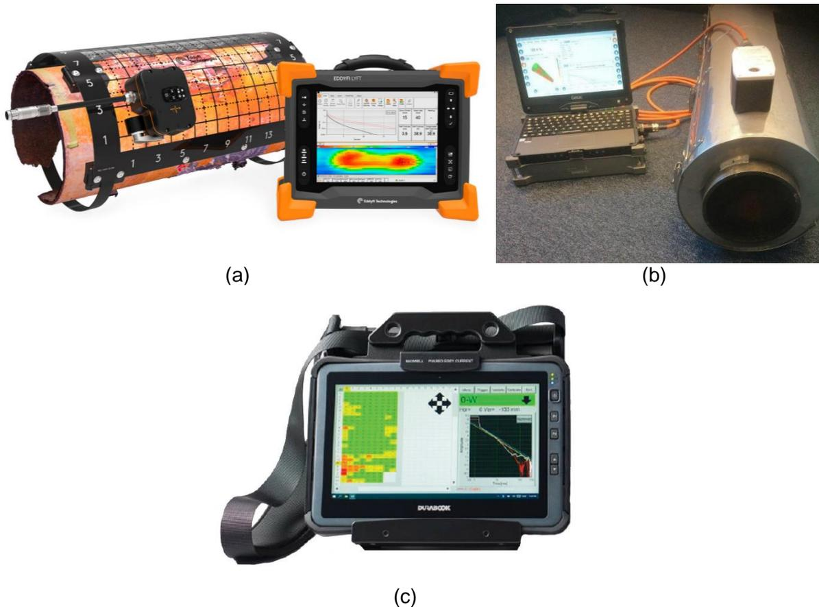
**Figure A2-32: Equipment for pulsed eddy current inspection: (a) Lyft (courtesy of Eddyfi), (b) Sonopec (courtesy of TUV Rheinland Sonovation) and (c) PECT (courtesy of Maxwell NDT)**
