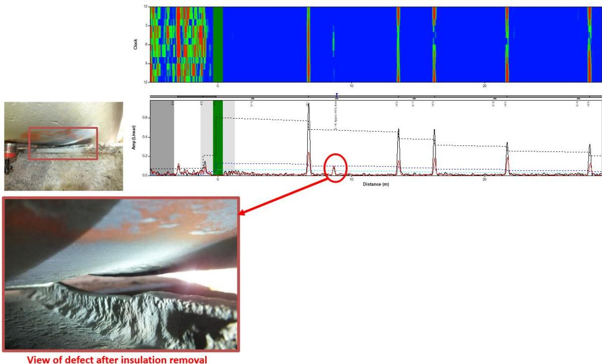
**Figure 8-7: GWT data (top) and corresponding area of corrosion at a pipe support (bottom), confirmed after removal of the insulation and lifting of the pipe off the support.**
