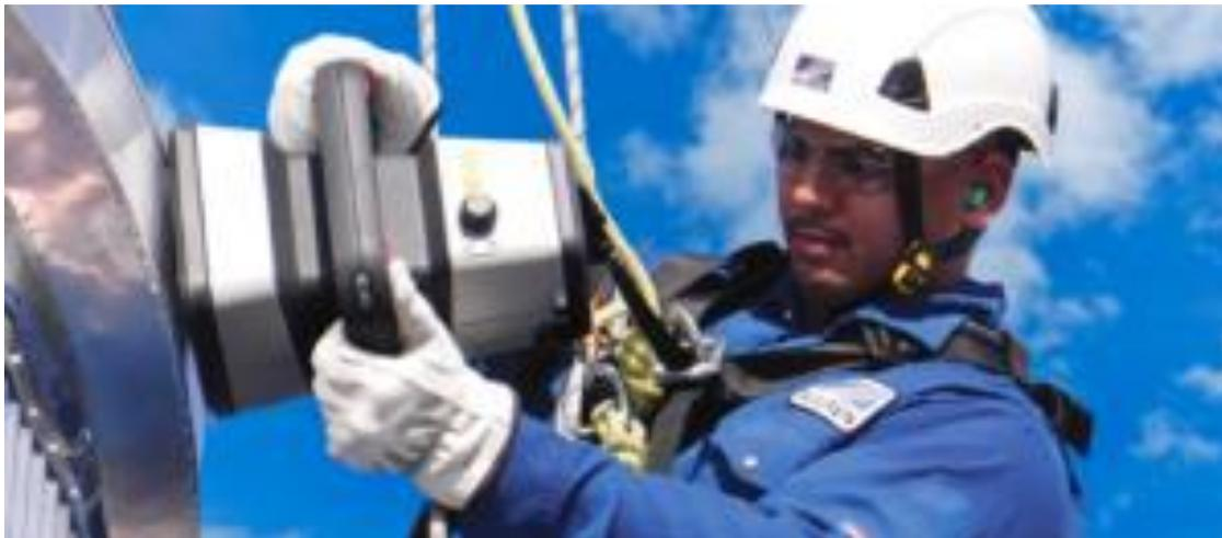
**Figure A3-1** Acuren's MDI equipment for moisture identification (courtesy Acuren)
