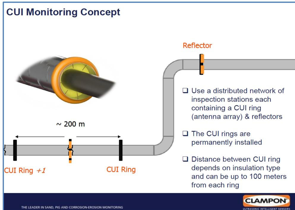
**Figure A3-7 Concept of the Guided Microwave system from ClampOn (courtesy ClampOn)**
