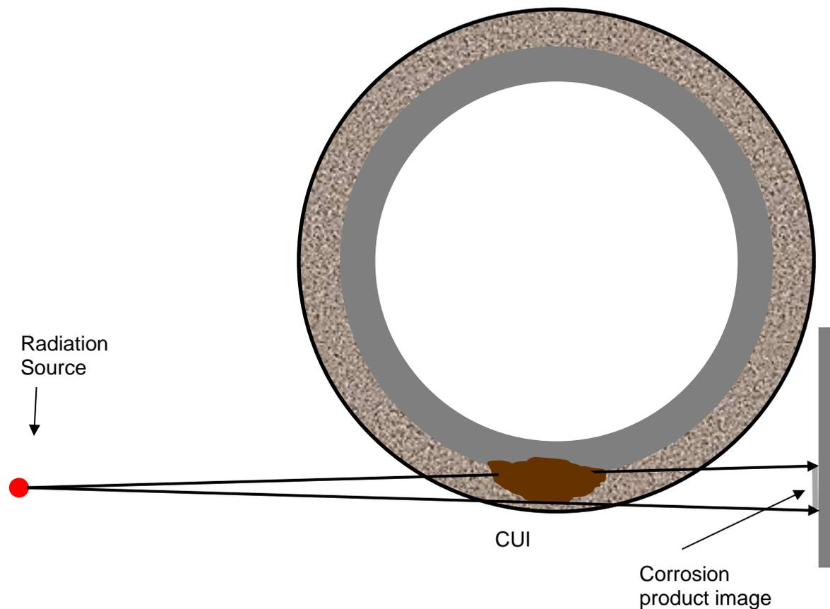
**Figure A2-19: Schematic of radiography of large diameter pipe showing image of pipe wall OD profile and any corrosion product associated with CUI.**
