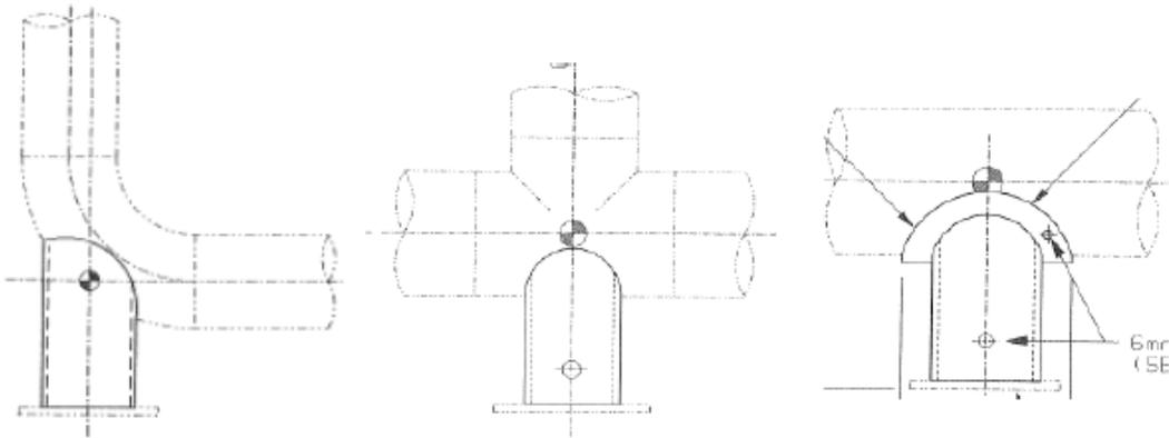
**Figure 4-2: Vertical trunnion on an elbow, on straight pipe/T-piece, trunnion on a straight pipe with reinforcement pad.**
