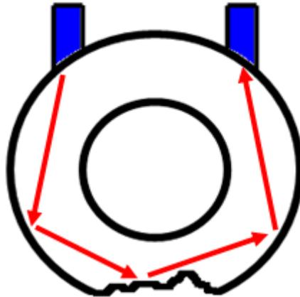
Figure A 1-11: Illustration of Verkade technique using circumferential inspection of a corroded area.
