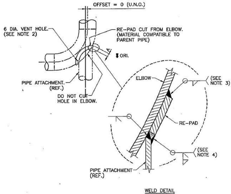
Figure 4-3: Vertical trunnion welded to elbow. With reinforcement plate around the trunnion. External surface of process pipe exposed inside trunnion.
