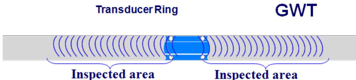
Figure A 1-1 Schematic of a long range guided wave system (courtesy Guided Ultrasonics Limited)
