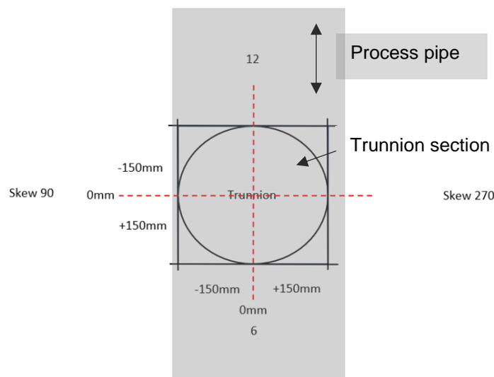
**Figure A 1-5: Medium Range Phased Array scan arrangement and nomenclature**
