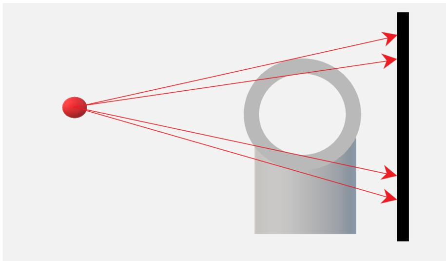
**Figure A 1-7: Principle of tangential radiography for inspection of small diameter pipes with trunnion pipe support.**
