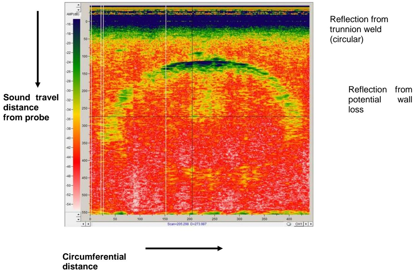
**Figure A 1-4: Example inspection result of a guided bulk wave system**
