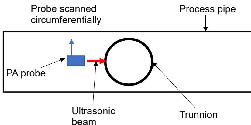
Figure A 1-2: Schematic of the long range PA method
