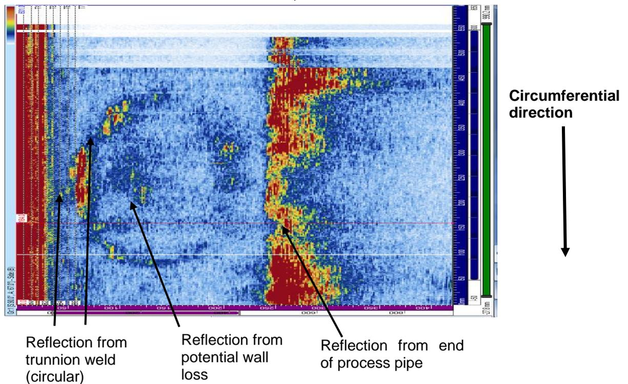
**Figure A 1-3: Example results from short length of process pipe with trunnion. Scan data shows reflections from trunnion weld and potential wall loss as well as reflections from the end of the short length of process pipe.**
