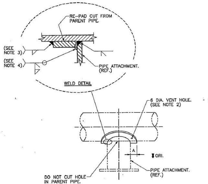
Figure 4-4: Reinforcement plate ring around vertical trunnion on straight pipe. Process pipe external surface exposed inside trunnion.
