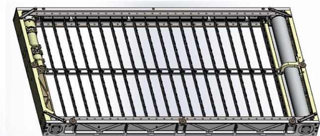
Optional baffle design fits inside belt arrangement and is recommended for vertical orientations where surface IR must be rejected. Baffle angle can be customised and fixed in place.
