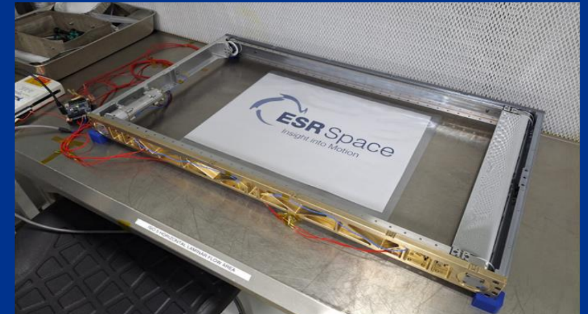
Breadboard Model LTS Build Completed April 2024 (End covers removed to show actuator and film spool)
