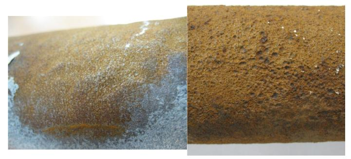
(a) (b) Figure 3. Two different forms of corrosion revealed after removal of the corrosion product (a) an even, undulating surface and (b) finely pitted surface.
