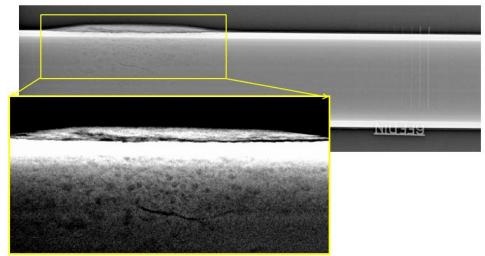
Figure 4. High pass filtered digital radiograph and magnified section with contrast settings optimised to show the fine pitting in the DWDI region of the image
