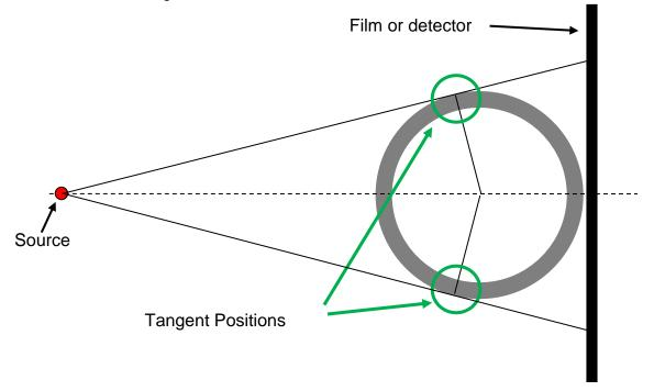
Figure 1. Setup for tangential (profile) radiography showing the tangent positions
