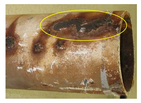
Figure 2. Corrosion scab under sized by ~1.5mm using tangential radiography
