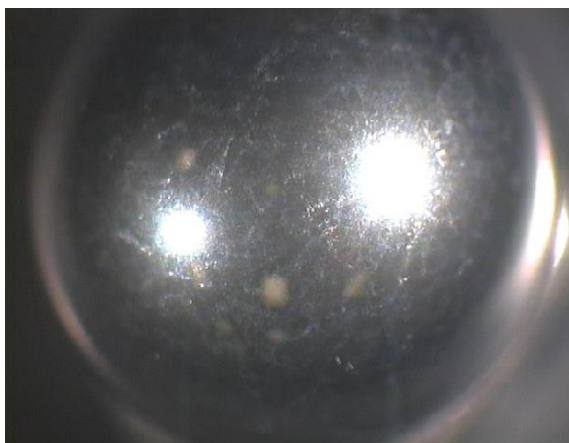
Figure 17. Ball from 1.50GPa contact stress test on lead, displaying lead mottles on surface. XRF analysis read ~100Å lead remaining
