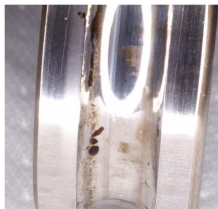
b) Showing black, degraded Z-type PFPE oil on the inner race of a life-tested ball bearing
