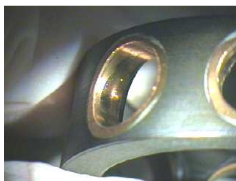
b) Lightweight hybrid cage: leaded bronze inserts in Vespel SP3 cage
