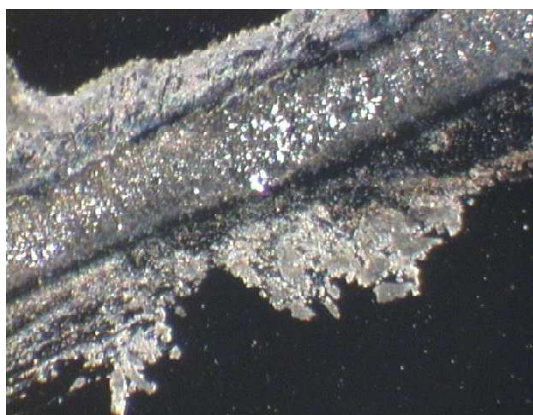
a) Showing build-up of translucent friction-polymer at edge of MAC-lubricated (Nye 2001a oil) wear track
