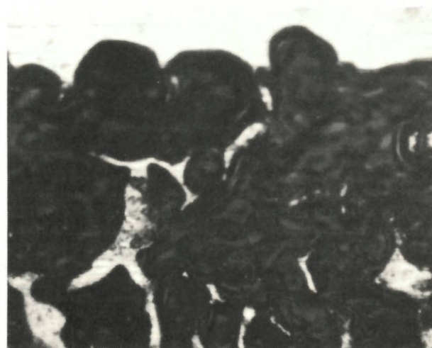
Figure 3d Inner race deposit
