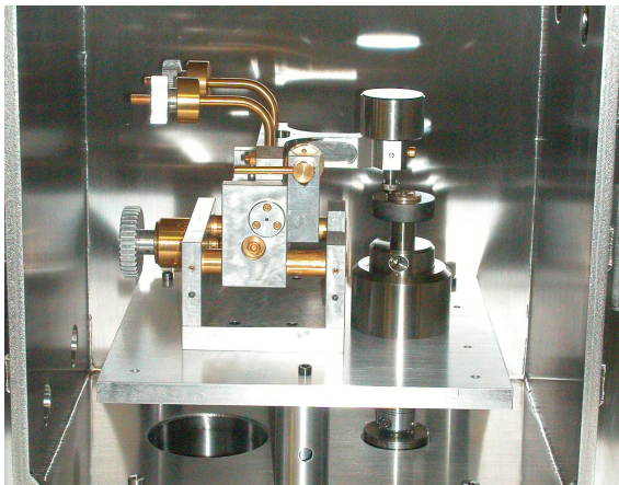
Figure 4. Vacuum pin on disc tribometer
