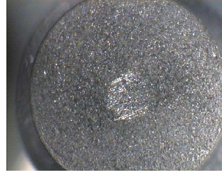
Figure 9. Wear scar after vacuum test
