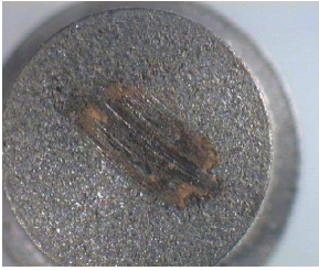
Figure 8. Wear scar after air test
