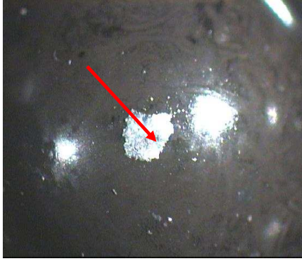
Figure 13: Compressed flake on ball surface indicated by red arrow. Note that the two other highlights are reflections from the microscope lighting
