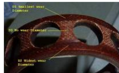
Figure 17: Cage different wear zones
