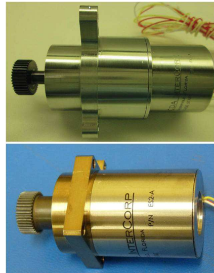
Figure 2: Pupil Wheel Motors – Enhanced Design (Top) and Original Design (Bottom)
