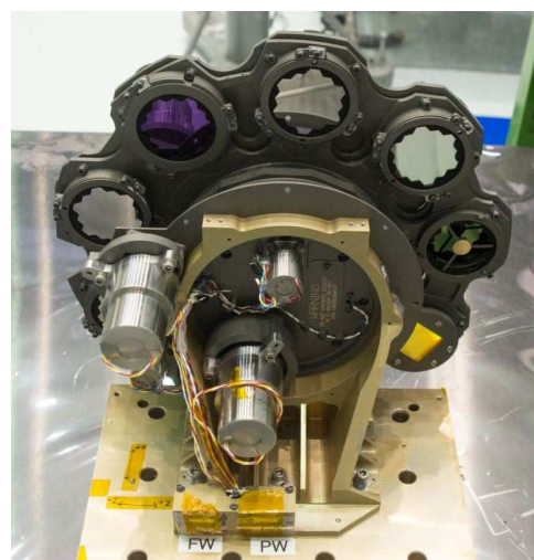
Figure 1: NIRISS Dual Wheel
