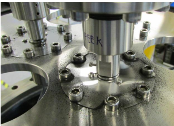
Figure 13. PEEK (centre) and Tecasint 1391 (left) bearing housings, displaying debris within test chamber
