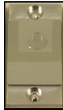
Figure 3. Oil drop enclosed by creep barrier boundary on a test plate.
