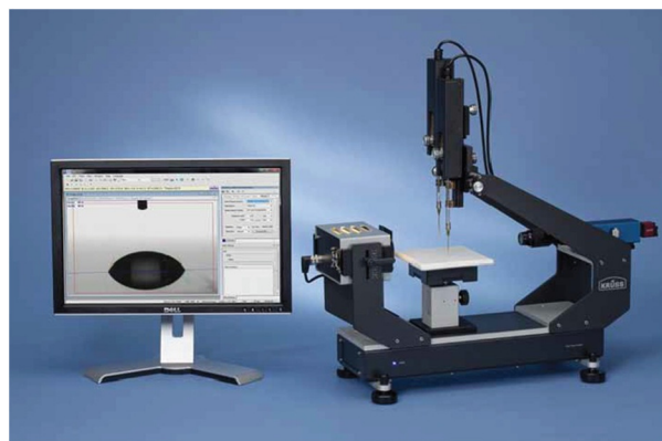
Figure 1. Krüss DSA25S drop shape analyser purchased by ESTL for contact angle measurements.
