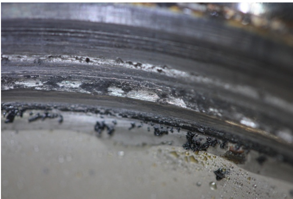
Figure 7. Showing wear on bore of flexspline
