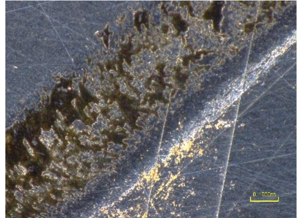
Figure 7. Very low R_a ( 0.010\mu\text{m} ) wear scar image showing extreme degraded oil
