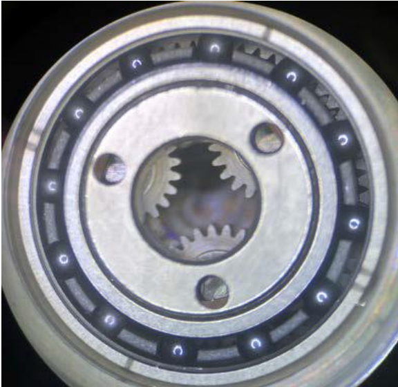
Figure 11 High Speed Stage Bearing in Very Good Condition Showing No Signs of Wear and Good Lubrication Coverage. High Speed Planet Gears Show No Presence of Wear Debris.
