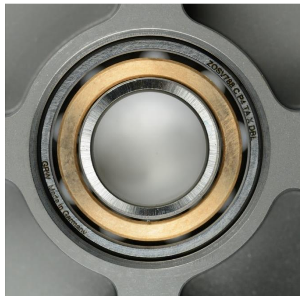
Figure 10 Floating Bearings (face-face) Following 80,000 Life Cycles.
