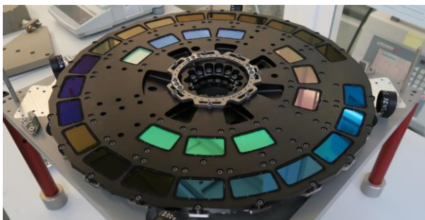
Figure 1. Filter Wheel Assembly (FWA)
