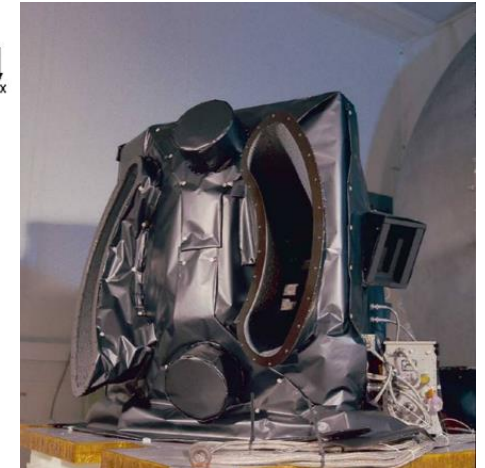
AATSR – its scan bearings were tested for 10^9 revs
