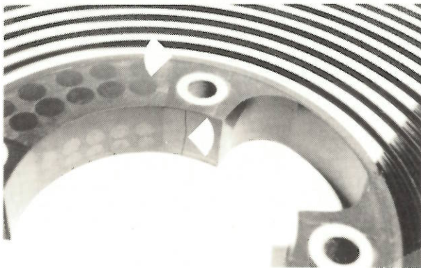
Figure 16. Cracked slip ring disc
