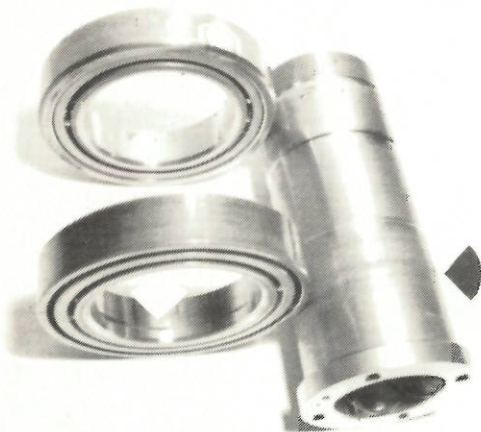
Figure 14. Shaft/inner race seizure.
