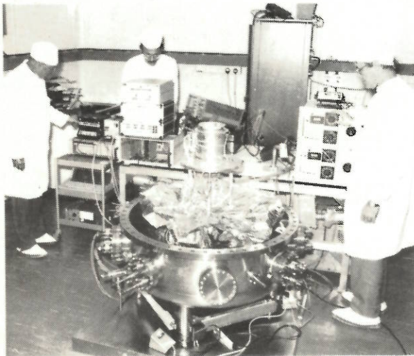
Figure 5. Giotto despin mechanism being installed in the ESTL 1-metre diameter test facility.
