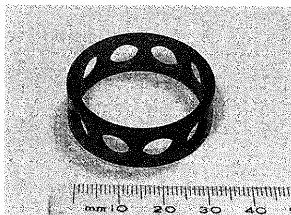
Fig. 3 SILICON CARBIDE CAGE, PRIOR TO COATING WITH \text{MoS}_2
