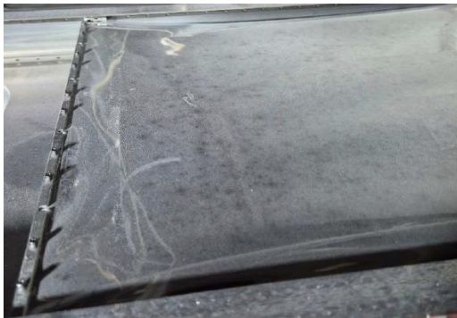
Figure 4-7 Thermal Film at the end of dust testing
