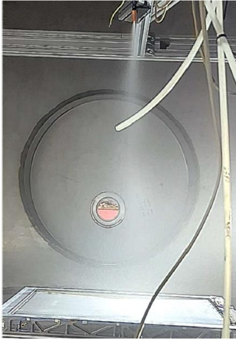
Figure 4-6 Dust Plume from Dust Exposure #4 (heavy)
