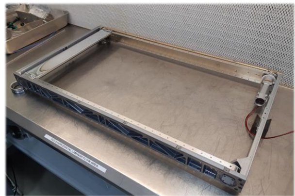
Figure 1-1 Breadboard Mechanism (with covers removed)
