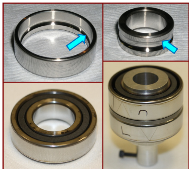
Figure 4. Angular contact bearings (FAG B7004), outer diameter 42 mm, inner diameter 20 mm, 11 balls 6.35 mm diameter, 15° free contact angle; Top-left and top-right, uncoated bearing outer and inner ring; arrows point to the up-to-coat surfaces (races); bottom-left, assembled bearing after races coating (steel spheres are encapsulated in a polymeric brown/grey PGM cage visible between the steel rings); bottom-right, couple of bearings mounted in back to back configuration, set for bearing-rig test.
